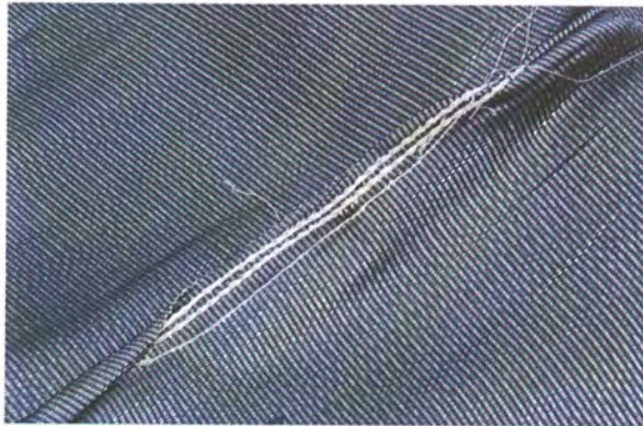
The seam of the fabric—3 15-ft.-wide fabric panels were sewn together to get the desired width of 45 ft. It was folded and rolled prior to shipping. The fabric rolls were attached to a 50-ft.-long spool. Photo courtesy of Triumph Geo-Synthetics.
