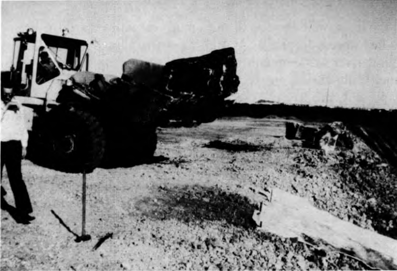
Fig. 13. Port Kembla Seawall, Australia: field tests on geotextile penetration resistance.
