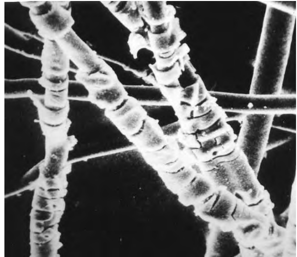
Figure-3 : Photograph of attacked geotextile by UV
