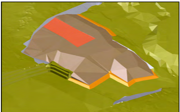
16. Filling of Cell 7
