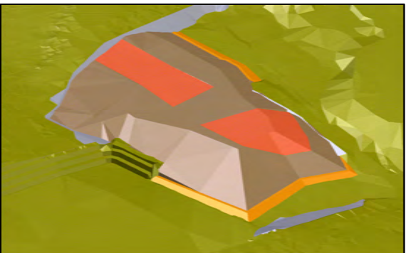
19. Infill between cells 7 and 8 and over Cell 7 to full landfill height
