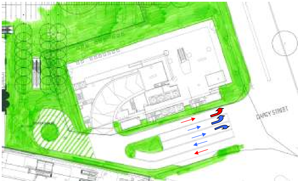
Figure 9 - Colston Budd Hunt & Kaffes Pty Ltd combined dive structure solution to access within Darcy Street (second revision, not the final plan, see Figure 10)
