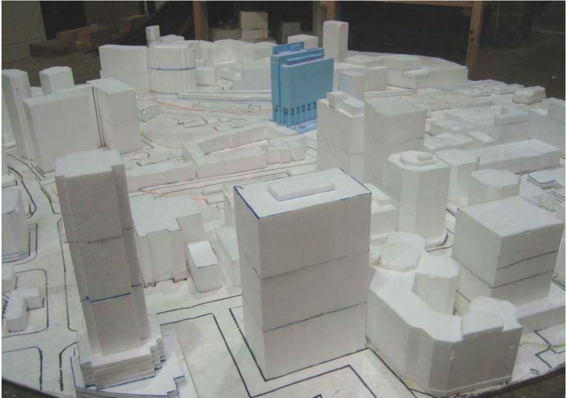
Figure 1b: Photograph of the Wind Tunnel Model (View from the North-East)
