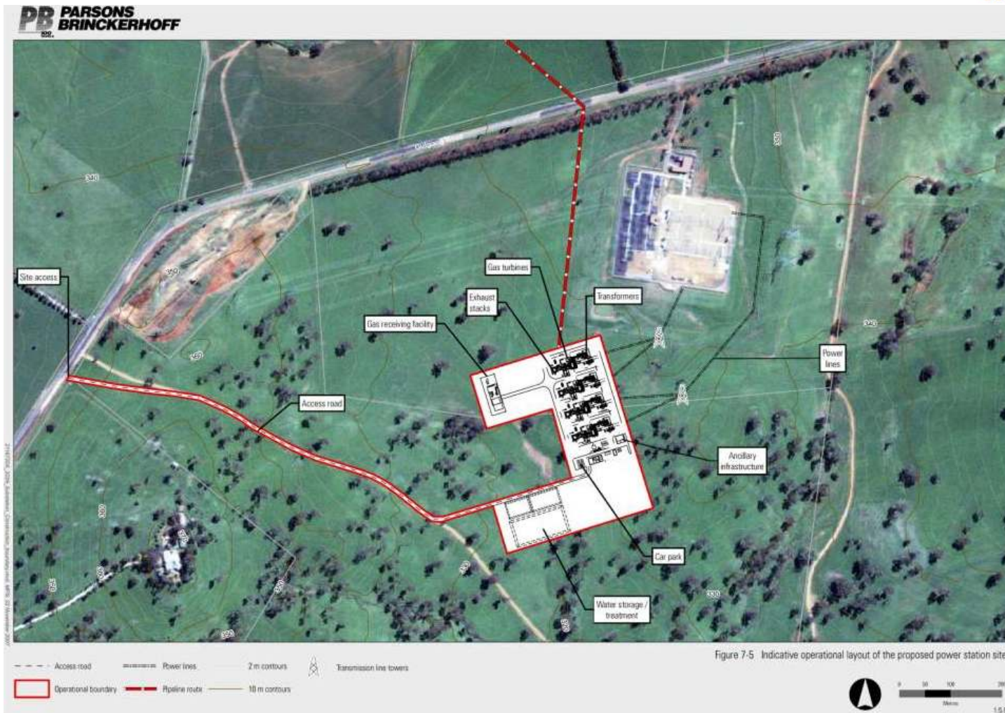
FIGURE 3.1: PRELIMINARY POWER STATION LAYOUT
