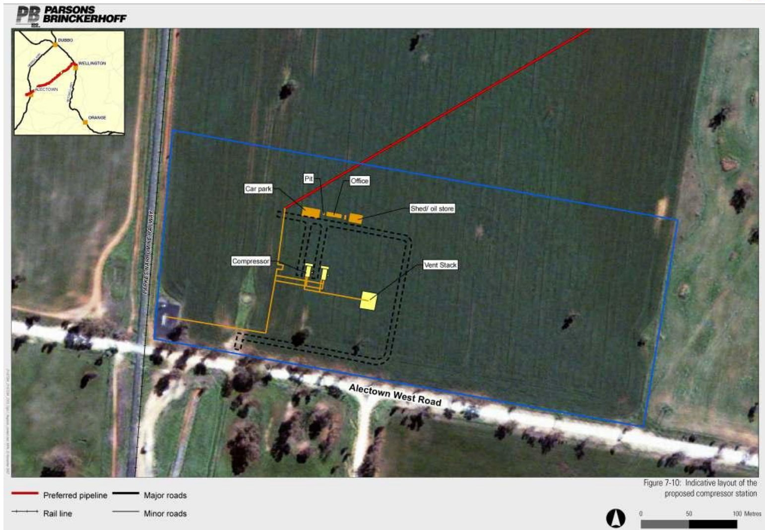
FIGURE 3.2: PRELIMINARY LAYOUT FOR OFFTAKE AND COMPRESSOR STATION
