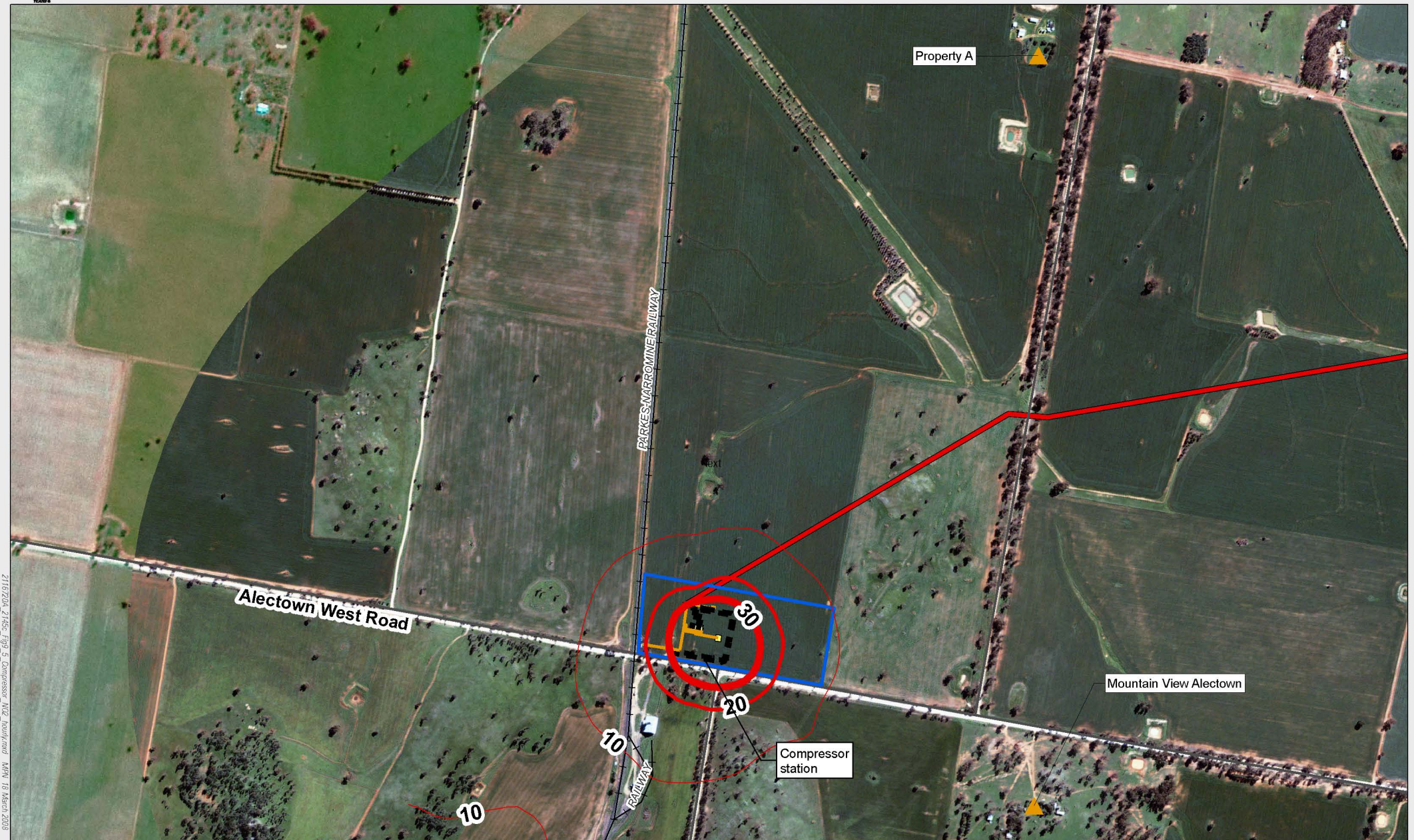
Figure 6-5 Maximum Predicted Hourly Ground Level NO x (as NO 2 ) Concentration ( \mu\text{g}/\text{m}^3 ) from the compressor
