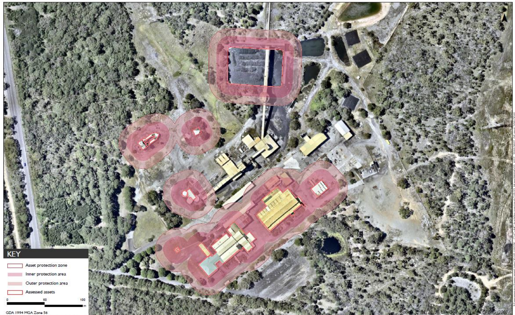
Figure 4. Location of asset protection zones
