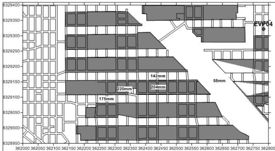
Figure 12 Key subsidence values projected onto the extraction plan (grey areas show extraction)
