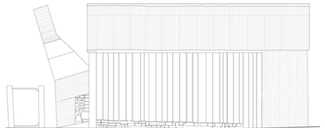
Figure 3.....Northern elevation of Workers Hut
