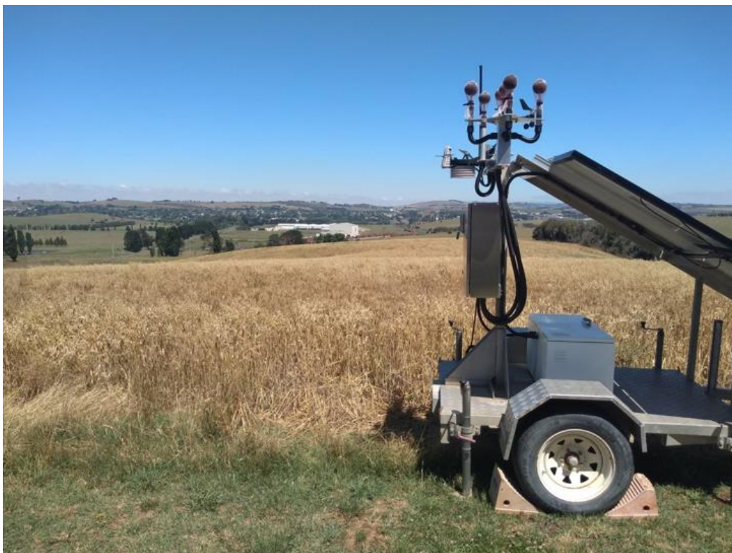
Plate 22 Noise monitoring trailer position at the time of the site inspection
