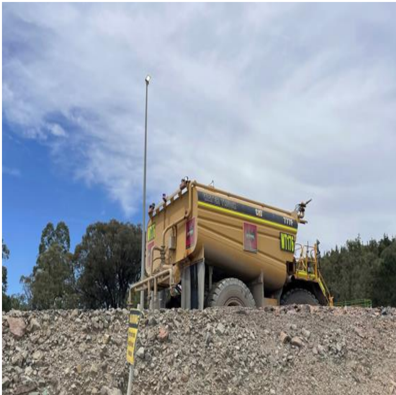
Plate 14 Water cart operating for dust control at South Waste Rock Dump
