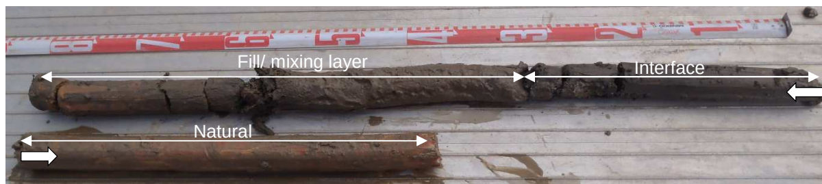
Photograph 1, shows undisturbed sample recovered from BH7B: 7.5m to 8.4m.
