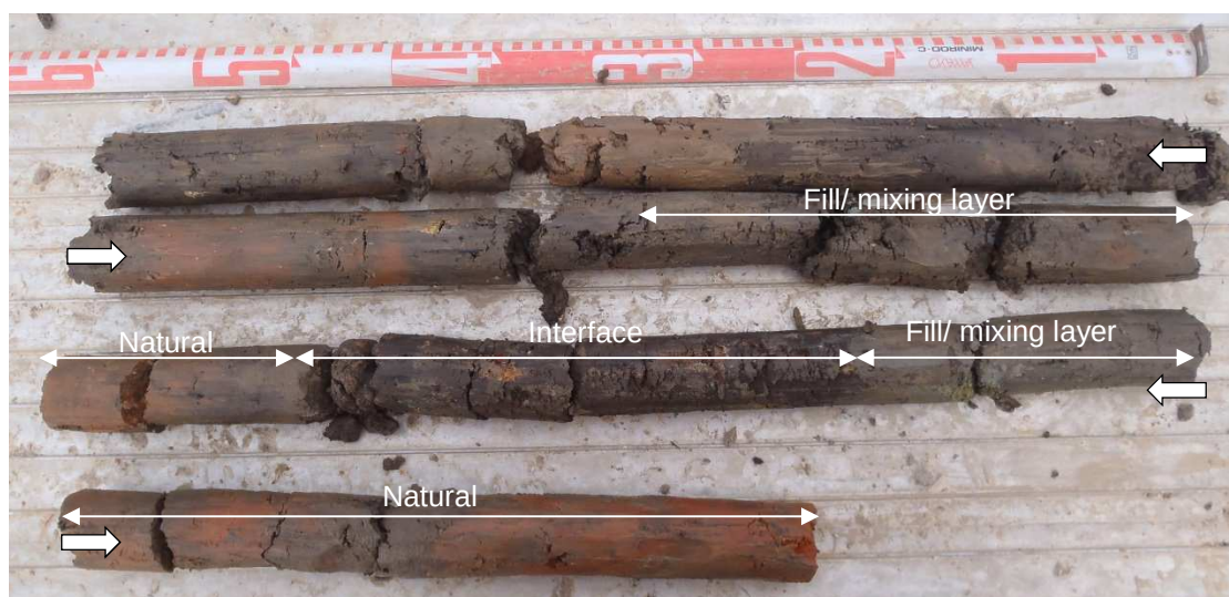
Photograph 5, shows undisturbed sample recovered from BH34B: 10m to 11.8m.
