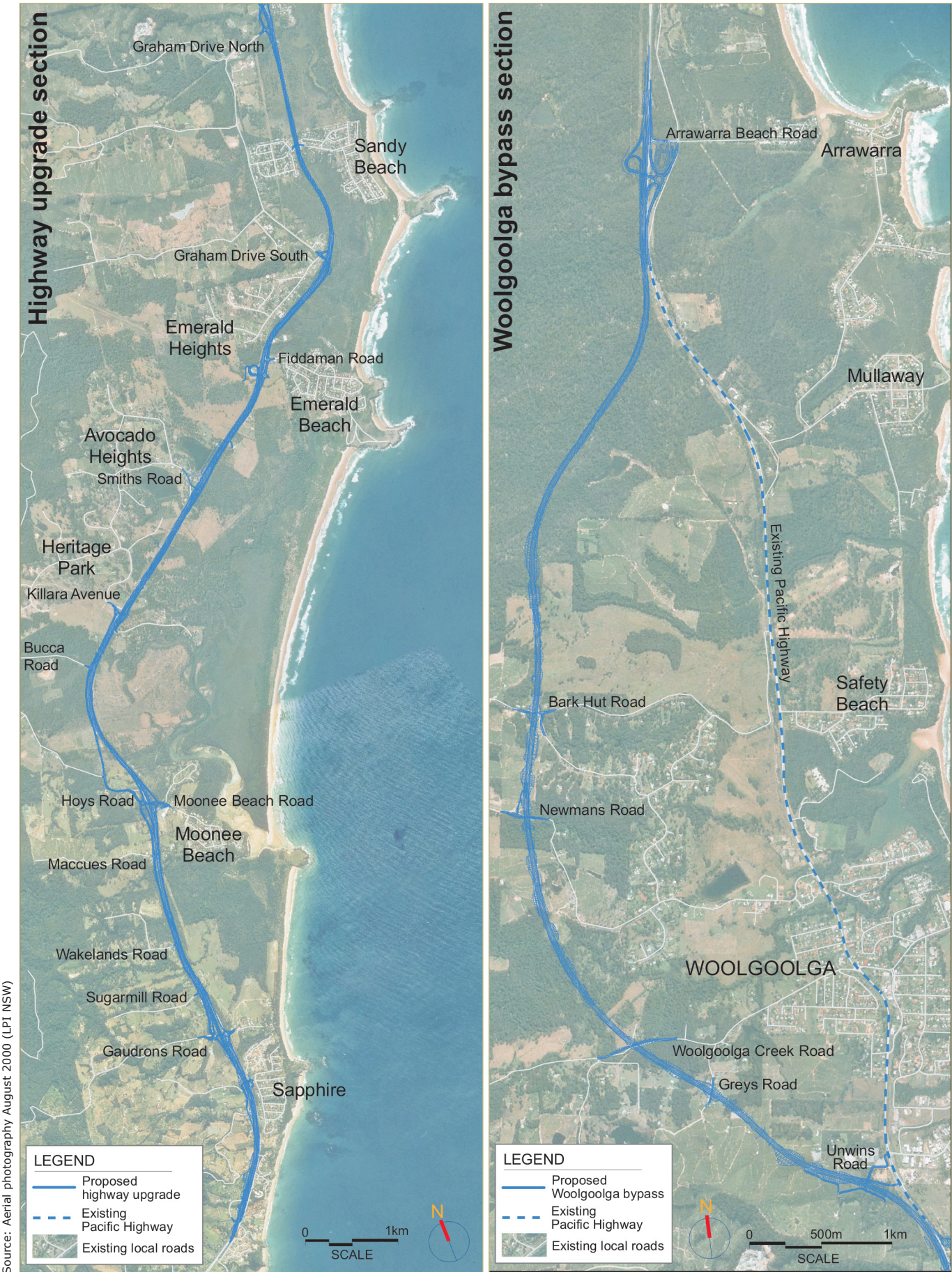
FIGURE 7.1 UPGRADE AND BYPASS SECTIONS OF THE PROPOSAL
