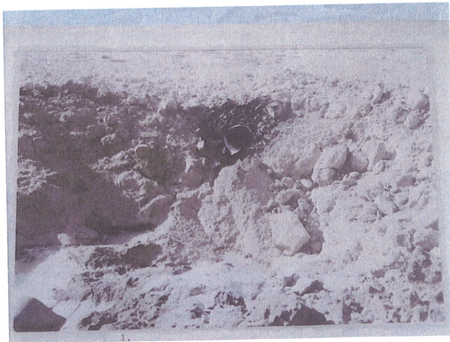
Explosion crater showing the down stream end of the fractured pipe
