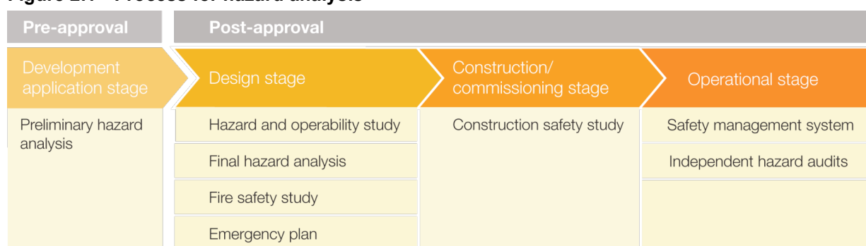
Figure 2.1 Process for hazard analysis
