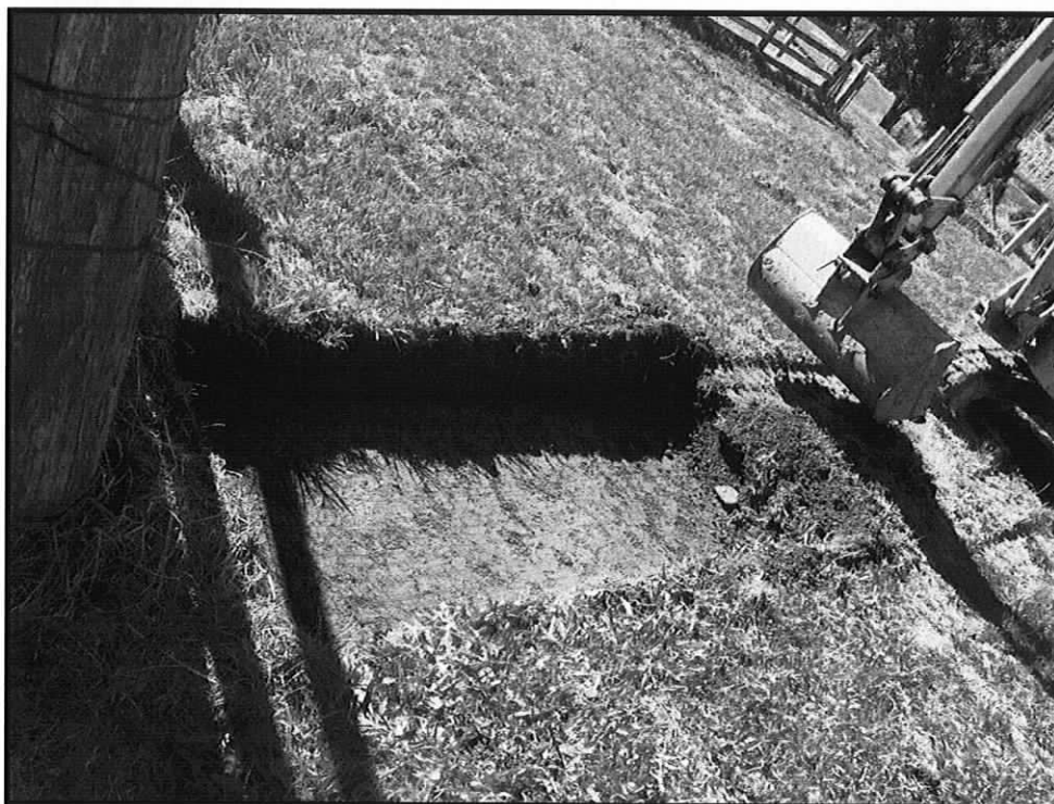
Plate 8. Typical test pit showing the basal clay unit (TP A2)
