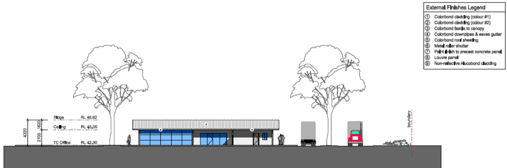
Transport Control Building - East Elevation
