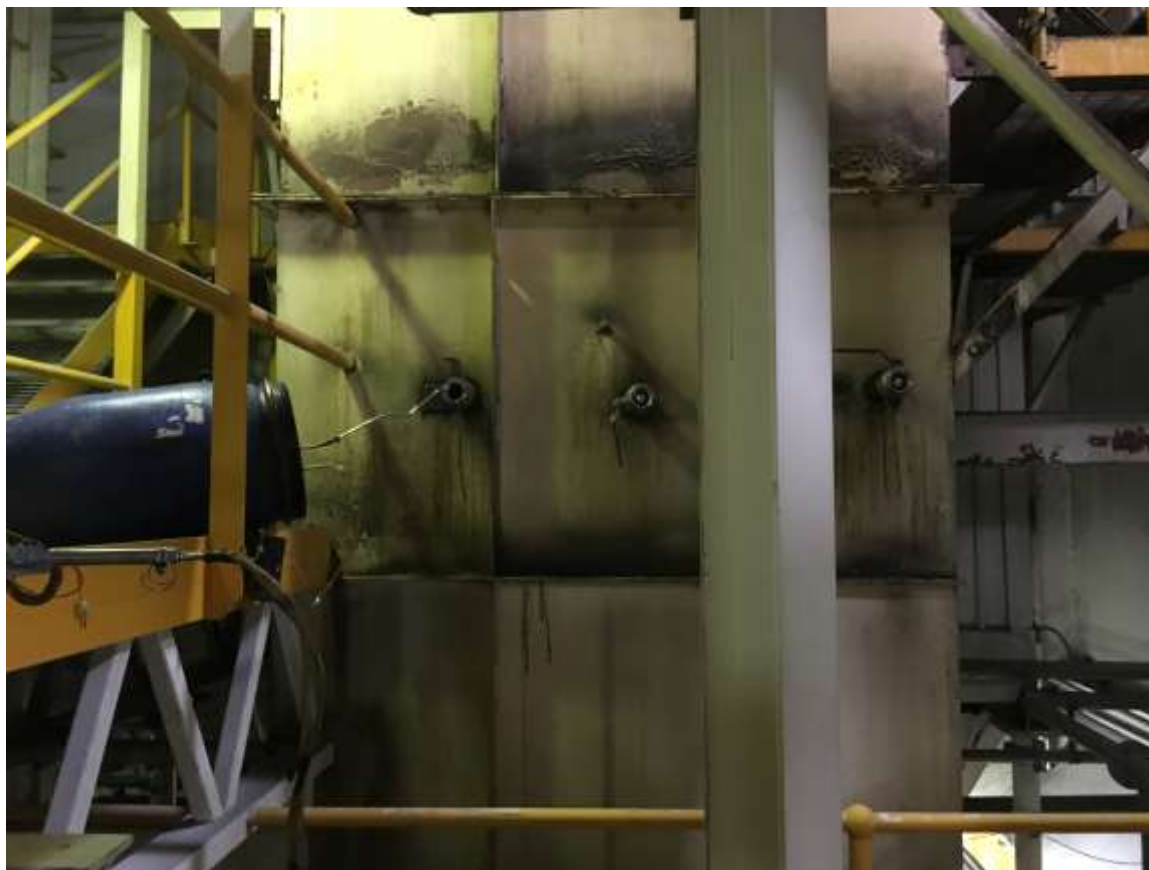
FIGURE D-6 GLUTEN DRYER NO. 3 – SAMPLE LOCATION
