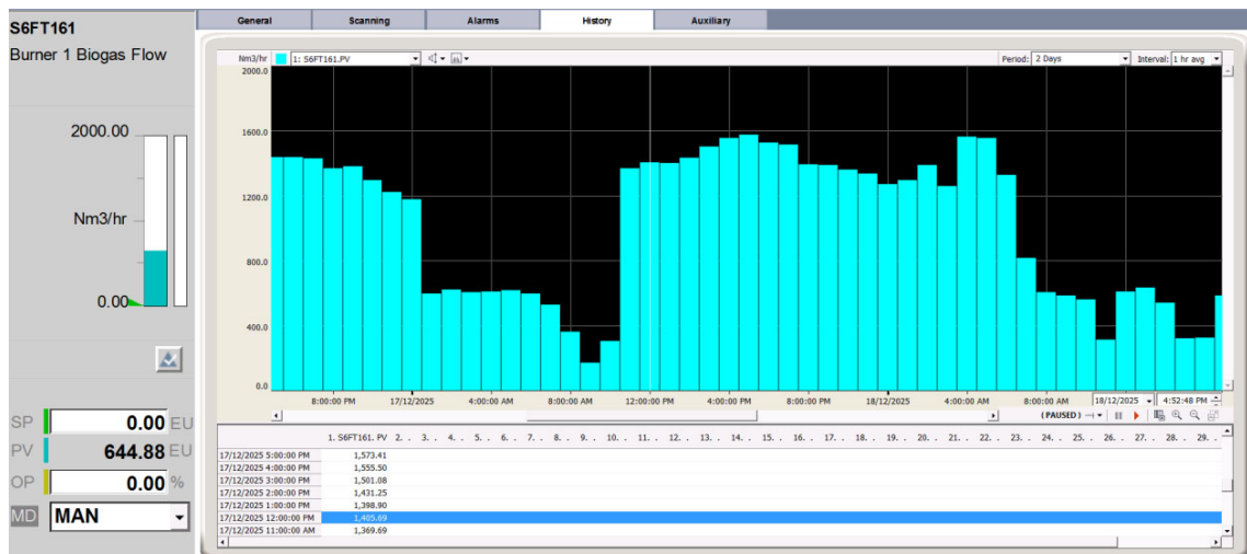
Figure 3: Plant Operating Conditions - EPA ID 35 - Boiler 6 Burner 1 Biogas Flow (17/12/2025)
