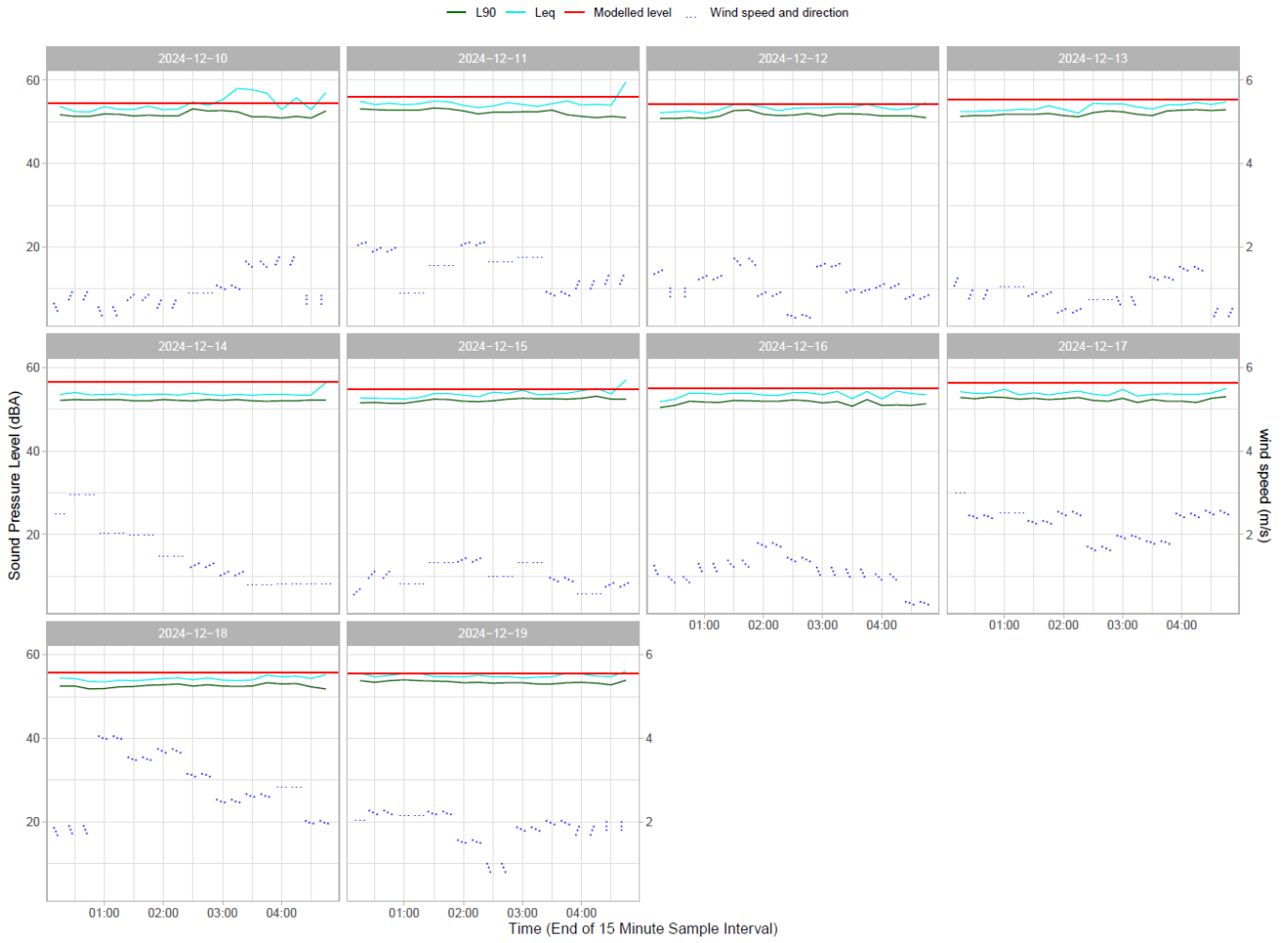
Figure B.5 Measured and predicted noise levels and wind conditions, Location 3
