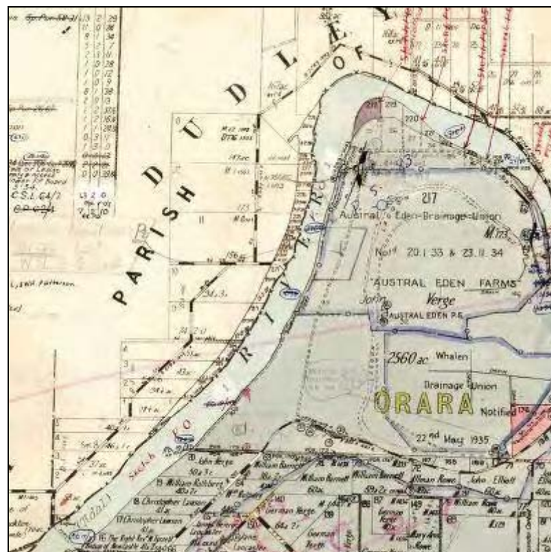
Figure 4.1 An example of how cadastral boundaries illustrate the erosion and accretion of the banks of the Macleay River. The top illustration is an excerpt from the Parish map of Cooroobongatti 1st Ed c.1886. The bottom illustration is an excerpt from the parish map of Kempsey, 8 th Ed 1954. Note the aggradation of the left river bank (and new portions on the new ground), and the corresponding erosion on the right bank.
