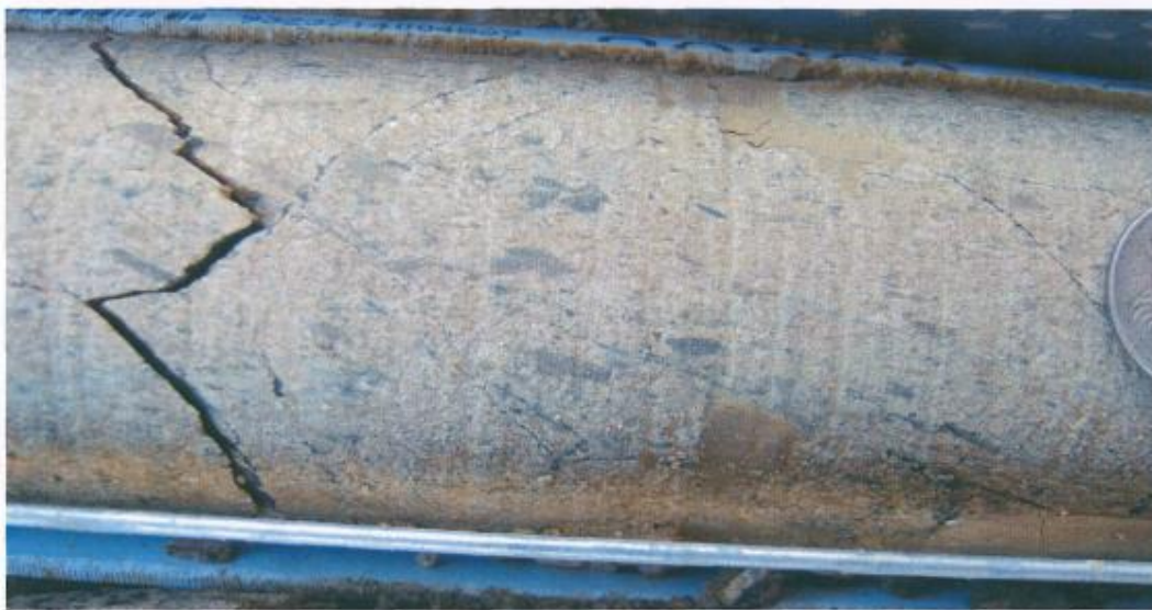
Figure 3: Slightly weathered mud chip greywacke at 13.4 m showing weak foliation defined by preferred orientation of elongate dark mudstone fragments.
