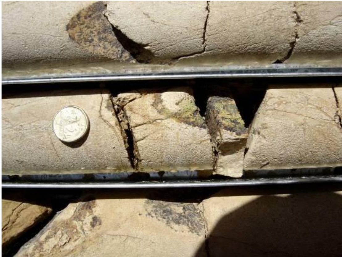
Figure 5: Weathered massive to weakly foliated greywacke, with prominent sub-planar fractures that are coated with brown iron oxide, black manganese oxide and a little yellow-green nontronite clay (centre). Coin is at approximately 8.7 m.
