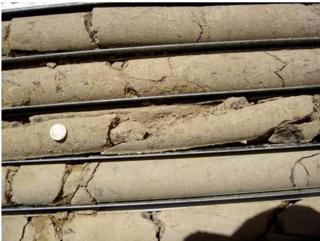
Figure 4: Weathered mud chip greywacke and greywacke with several sub-planar to irregular zones of fracturing and strong clay alteration (e.g. to the right of the coin and in the lower left of the image). Coin is located at 12.6 m.
