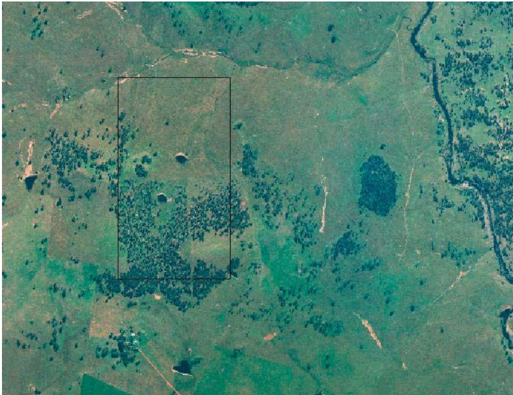
Figure 3: Aerial photograph of the landfill site and immediate surrounding area. The projected fault trace has been omitted, but it trends approximately northeast across the image from near the southwest corner to the northeast corner. The landfill site occupies much of the wooded area just left of centre. The image is approximately 2 km east-west. It is relevant to note that there is no topographic expression or photo-linear corresponding to the projected position of the fault.
