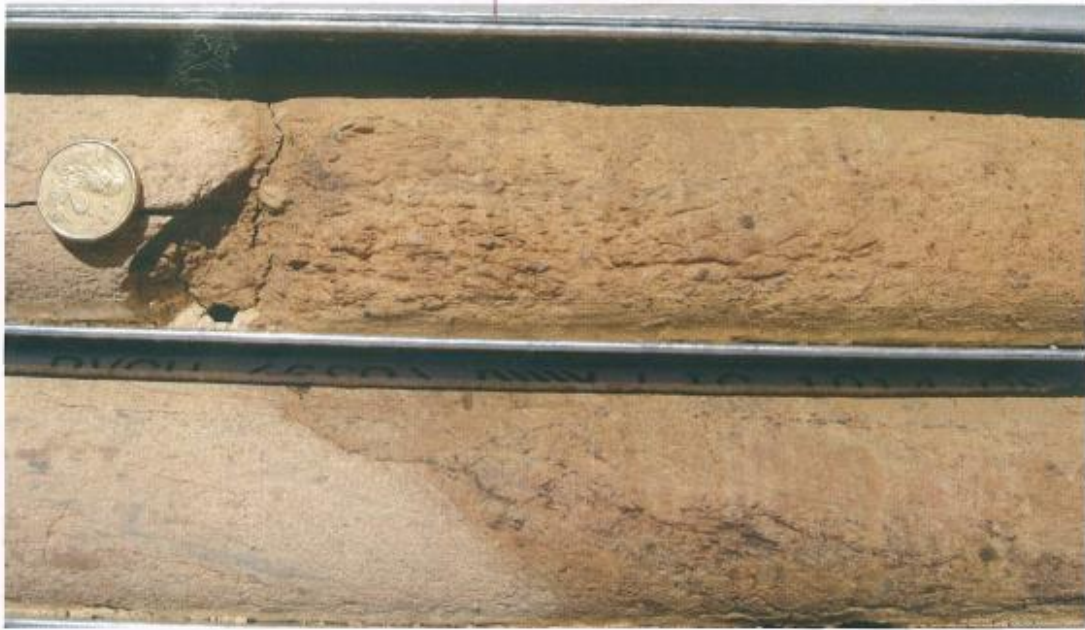
Figure 2: Weathered mud chip greywacke at 14.2 m showing zone of foliation to the right of the coin.
