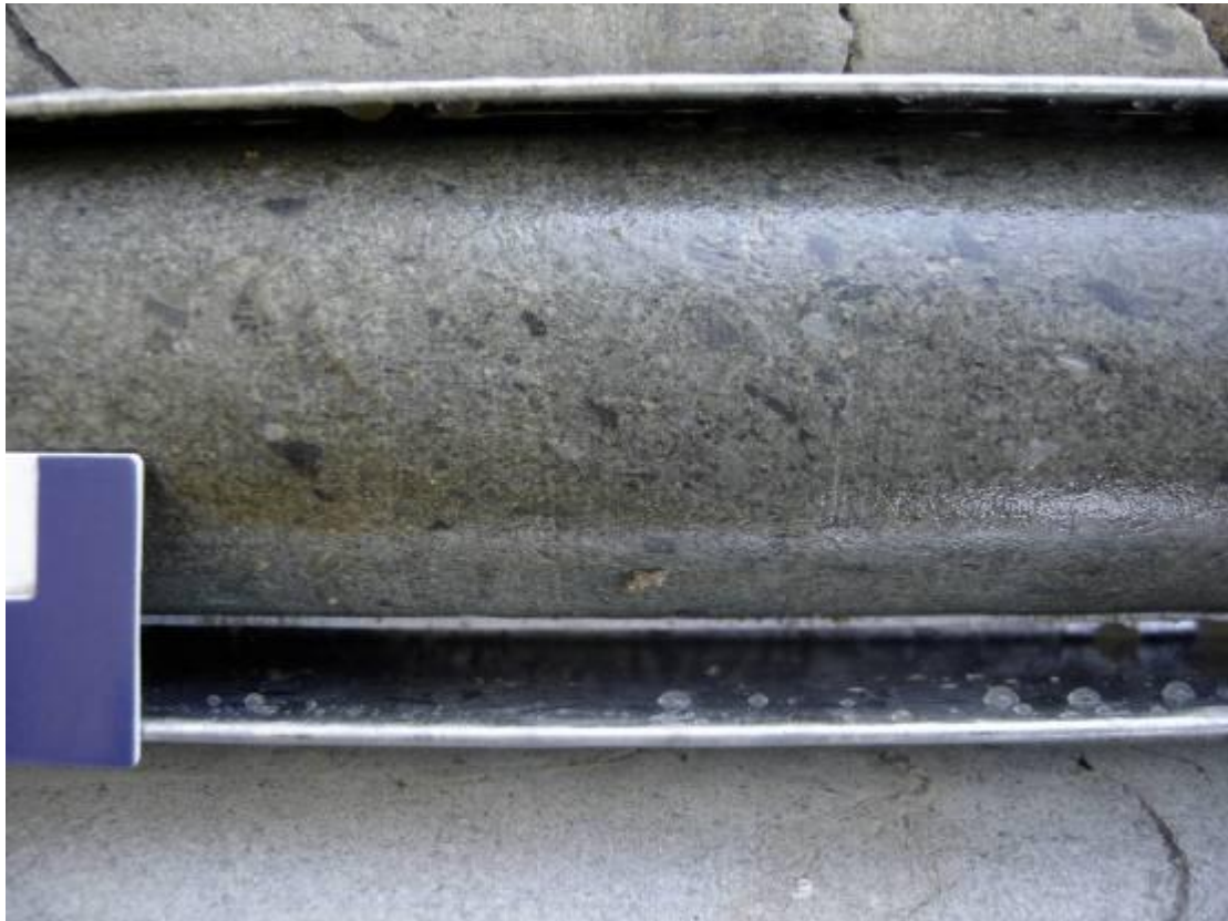
Figure 1: Fresh mud chip greywacke at 23.4 m. Dark fine grained angular to elongate mudstone lithic grains are enclosed in a medium grained greywacke matrix, in places containing a few slightly larger pale coloured quartz-rich grains. Blue scale on left hand side has centimetre markings.
