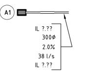
STORMWATER PIT, LINE & NUMBER INVERT LEVEL UPSTREAM
