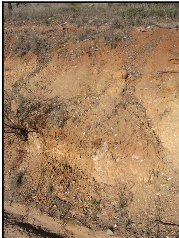
Plate 3: Yellow Duplex at Site 10, displaying duplex soil profile.
