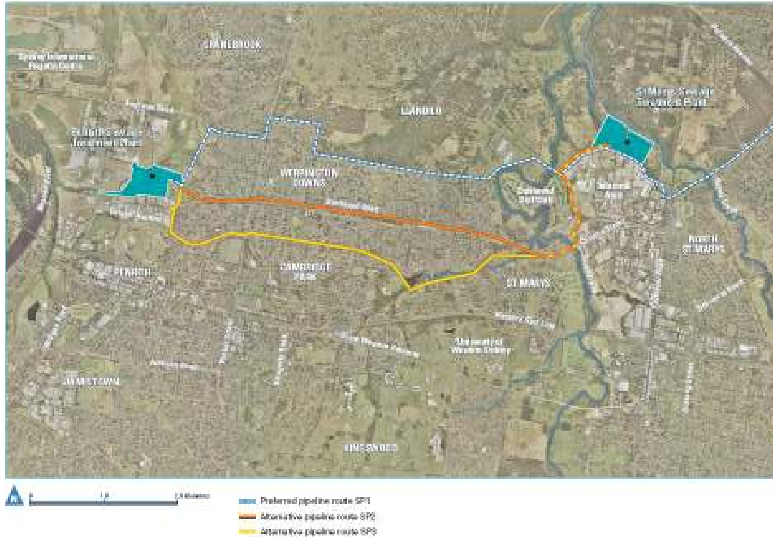
Figure 11: Alternative Routes Considered for the Transfer Pipeline between St Marys STP and Penrith STP
