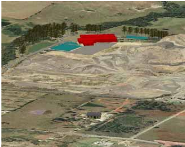
Figure 7.9: Predicted Visibility from Property E During Landfill Operation
