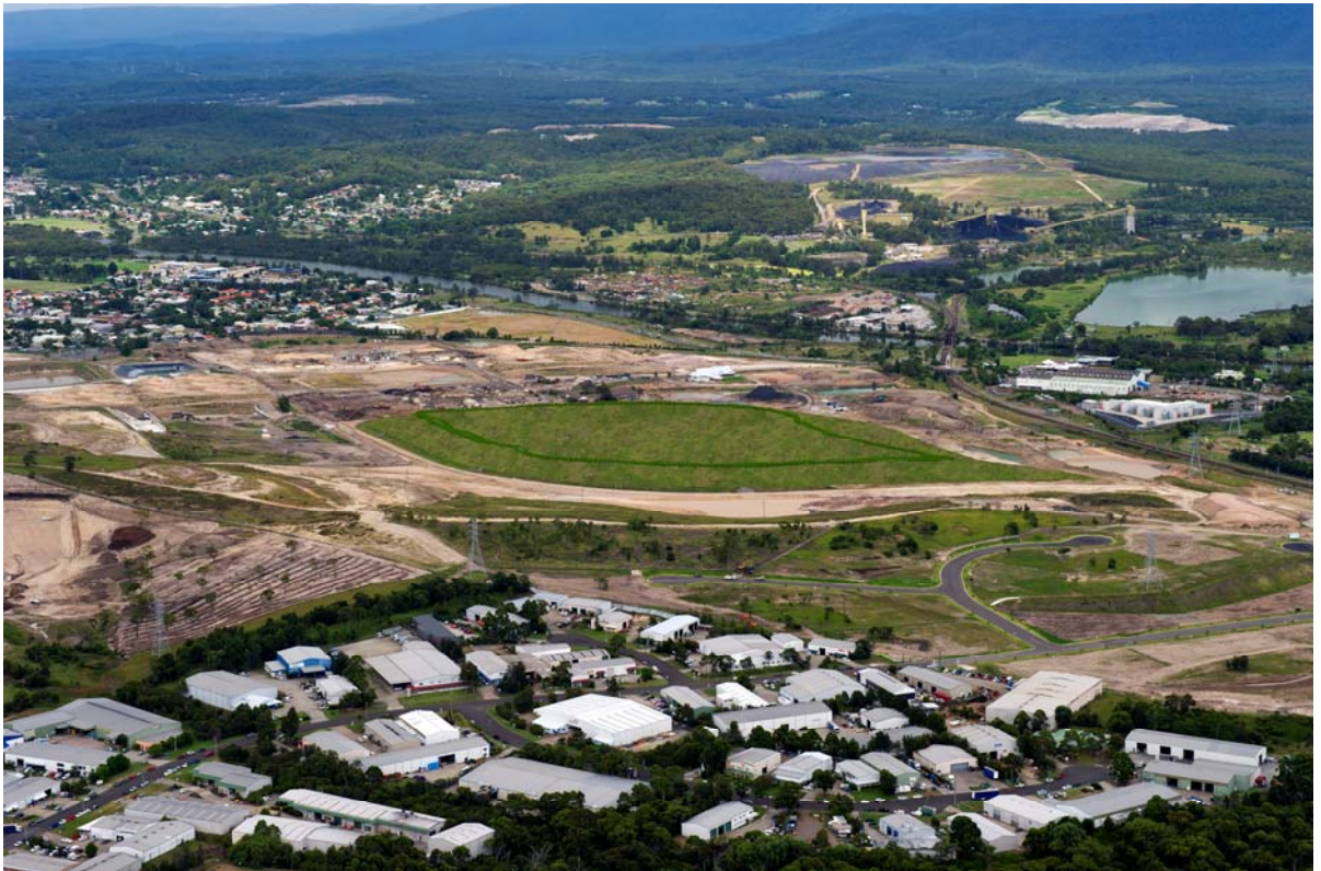
Photo 8C: Aerial photomontage of a single containment cell from the north-east, with height of cell raised by approx. 4m (to RL 38), with landscape cover over cell and slopes. Usable open space delineated by proposed ring of vegetation.
