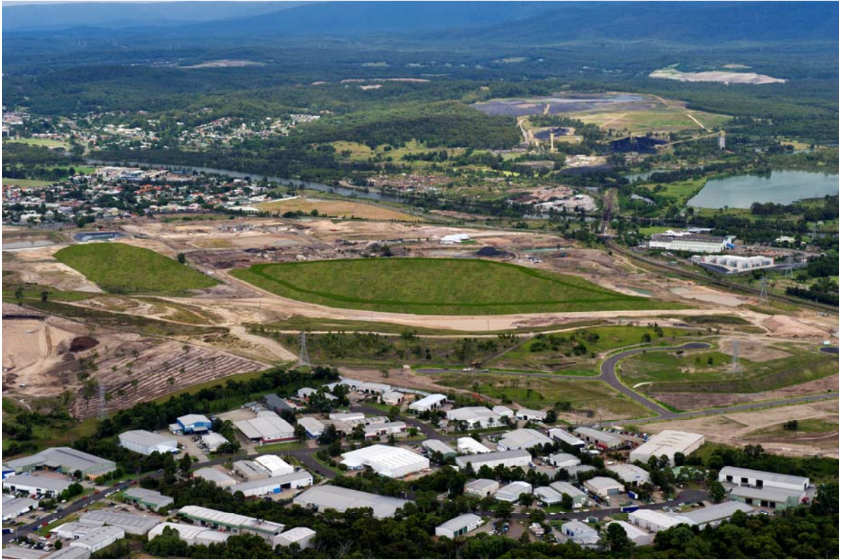
Photo 8B: Aerial photomontage of the proposed PCCS and IFL containment cells from the north-east, as approved, with usable open space at the top of the cell delineated by the proposed ring of vegetation.
