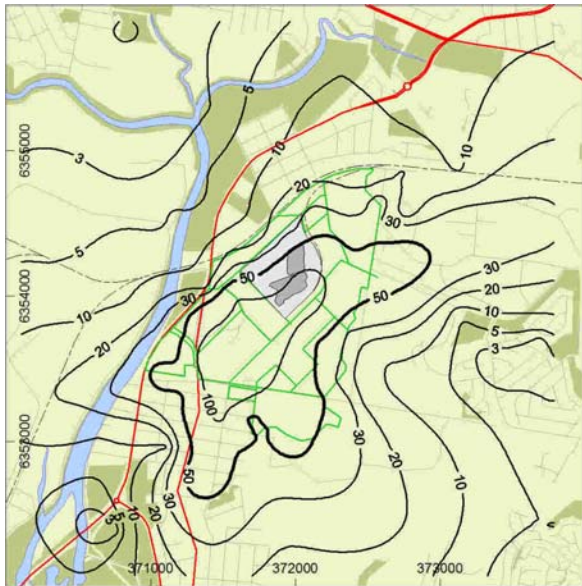
Maximum 24-hour average PM 10 - \mu\text{g}/\text{m}^3
