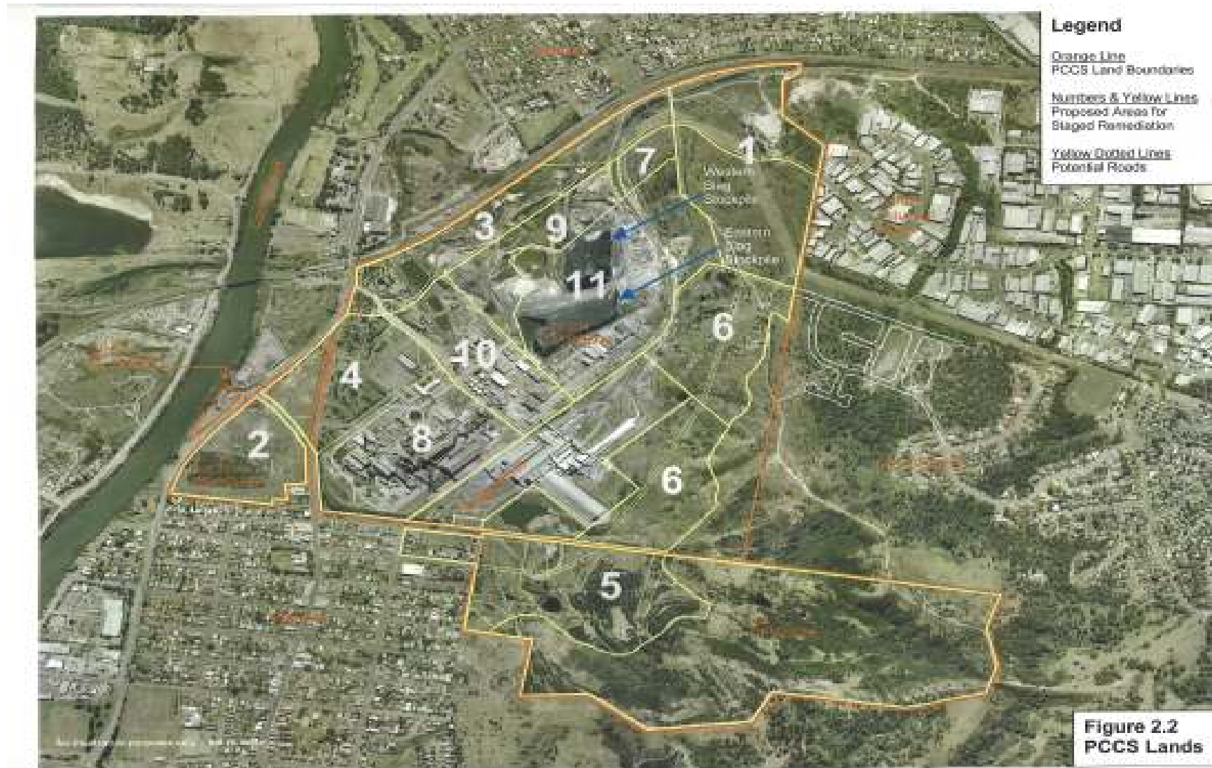
Figure 1 - Site Location (Site Boundary (Orange Line), Remediation Stages (Yellow Lines), Containment Cell Location (Areas 9 and 11))
