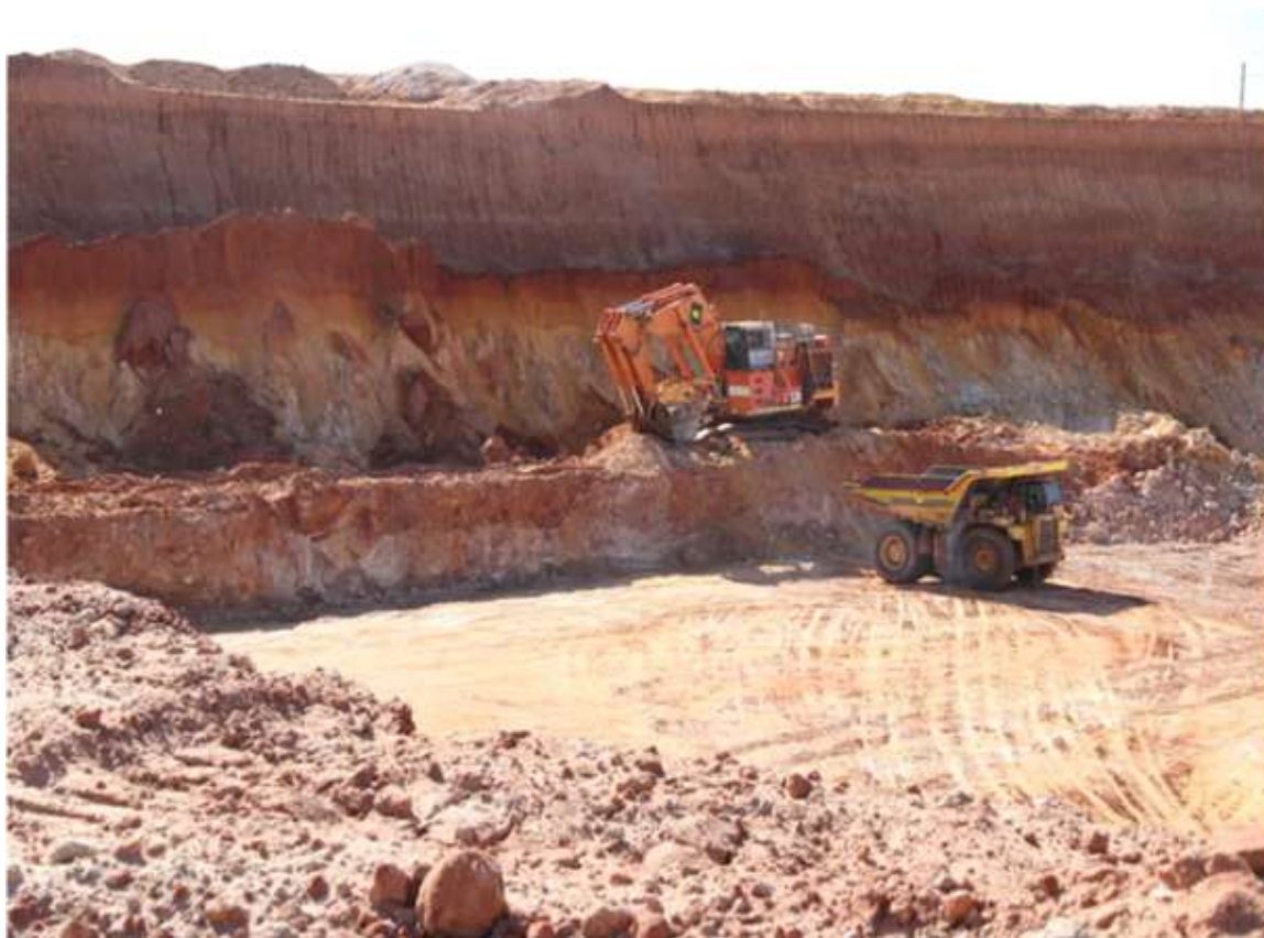
Overburden being removed by truck and shovel
