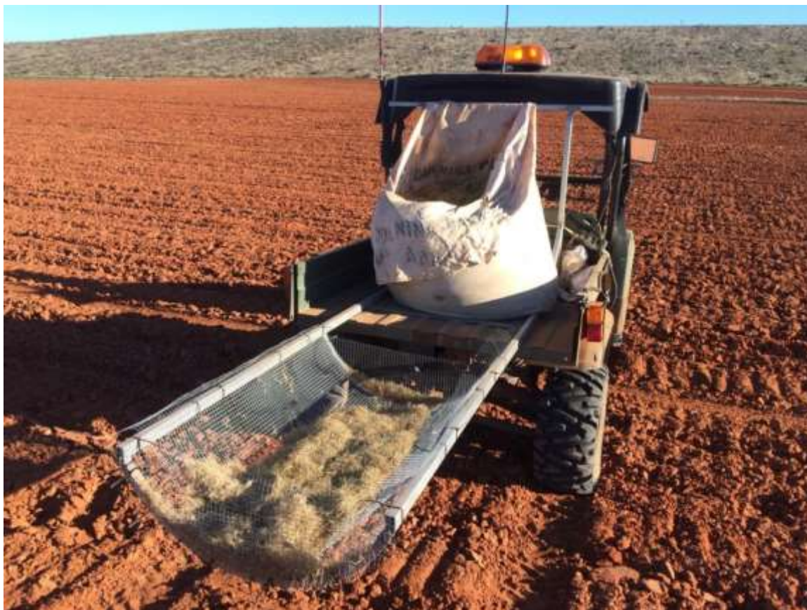
UTV with grass seed broadcaster attached to rear
