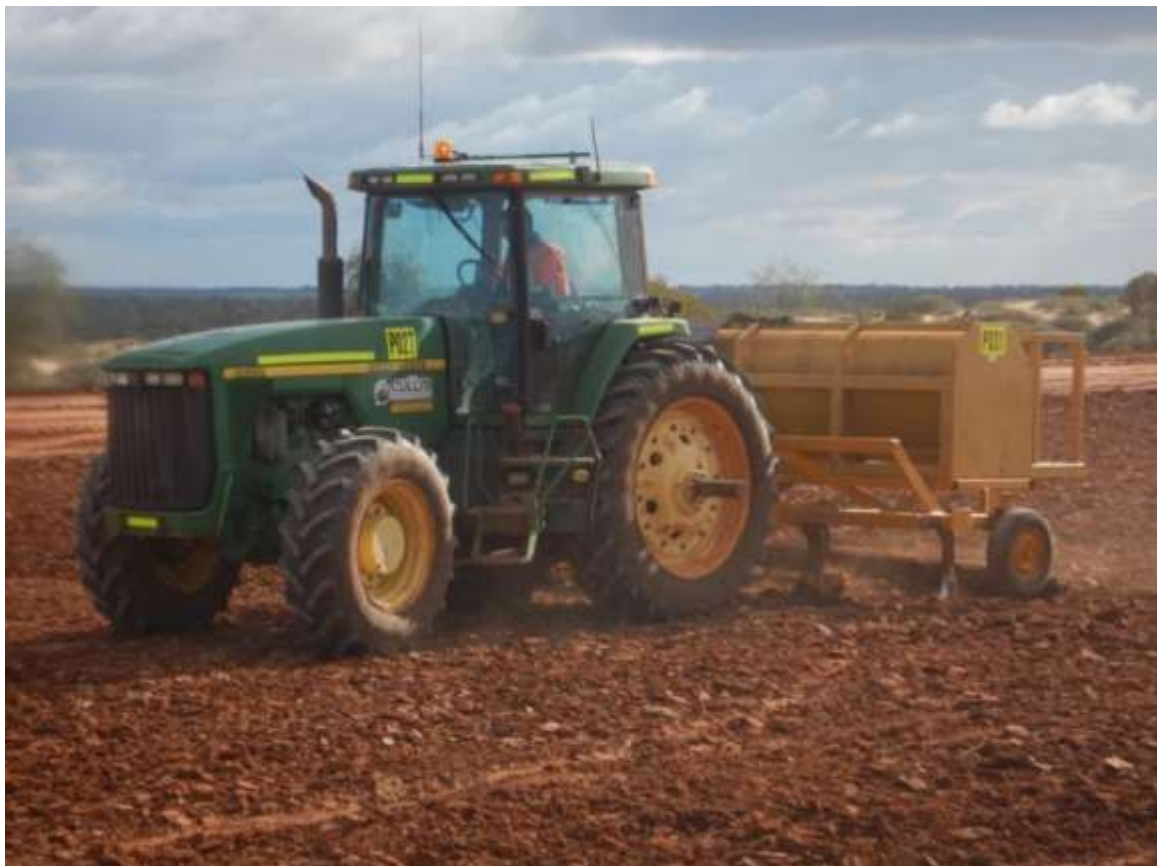
John Deere tractor with 5 tine plough and Gessner drum seeder mounted.
