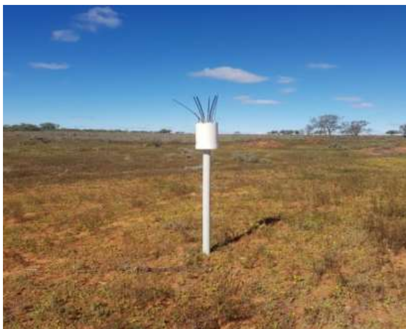
Dust deposition gauge at Manilla homestead
