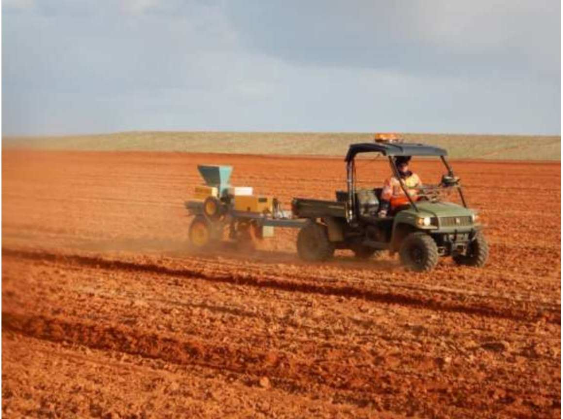
Burford tree seeder being towed by the UTV.
