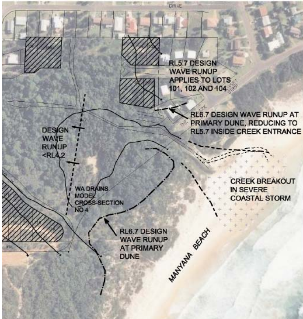
Figure 4.10: A summary of GBAC's coastal hazard inundation assessment. Source: gbaCoastal, June 2010.
