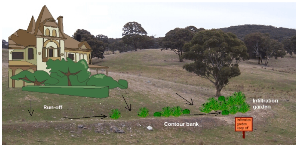
Figure 7 - Infiltration contour bank. Diagrammatic only.
