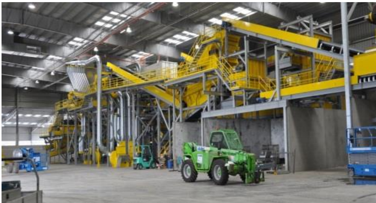
Figure 5 – View of plant inside the MPC (from the southern end) showing the conveyors which are electric-driven
