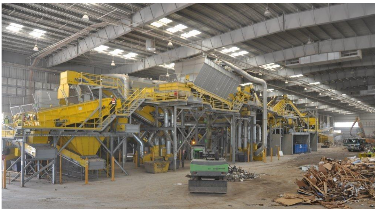
Figure 5 – View of plant inside the MPC (from the southern end) showing the conveyors which are electric-driven
