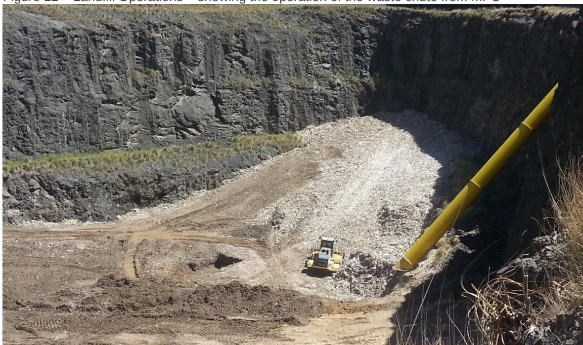
Figure 12 – Landfill Operations – showing the operation of the waste chute from MPC
