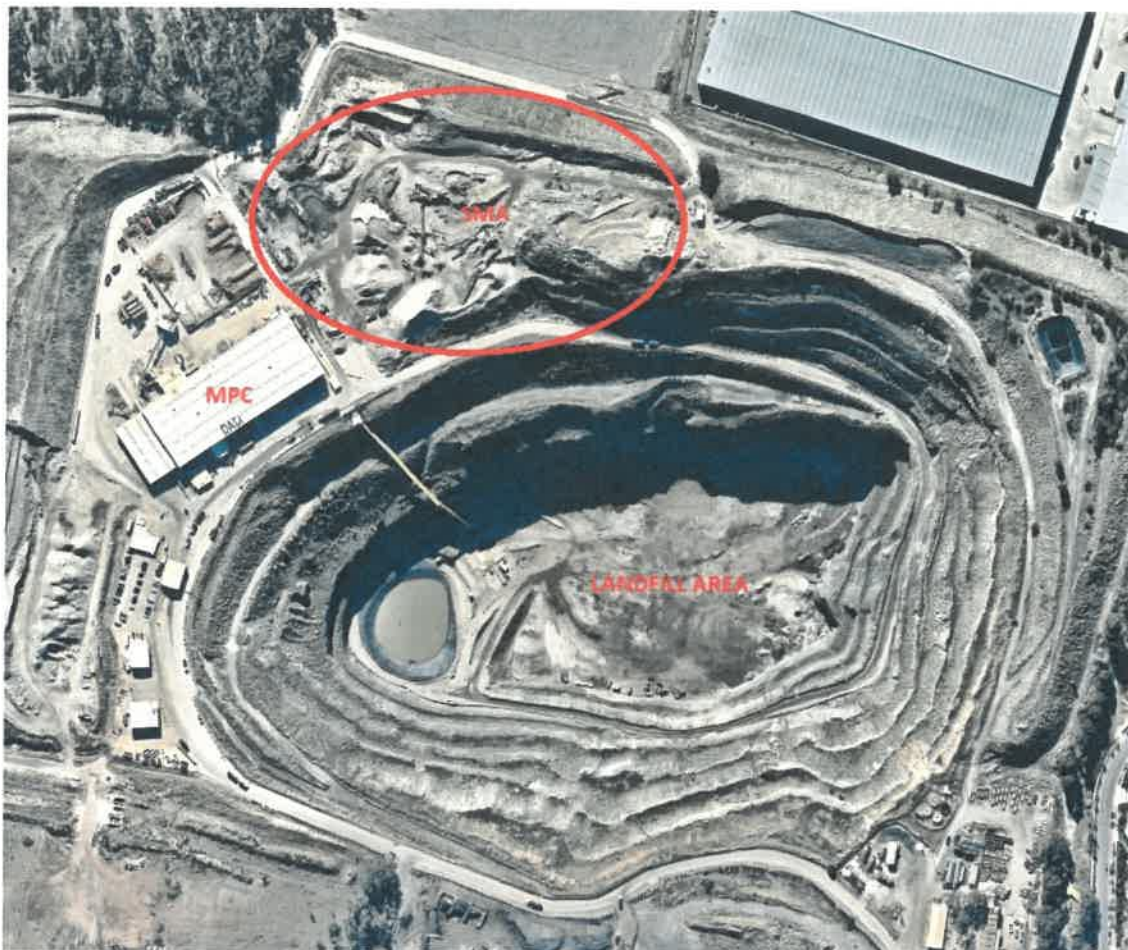
FIGURE 1 – Depicts the existing site layout and operational areas including Segregated Materials Area (SMA), Materials Processing Centre (MPC) and Landfill.
