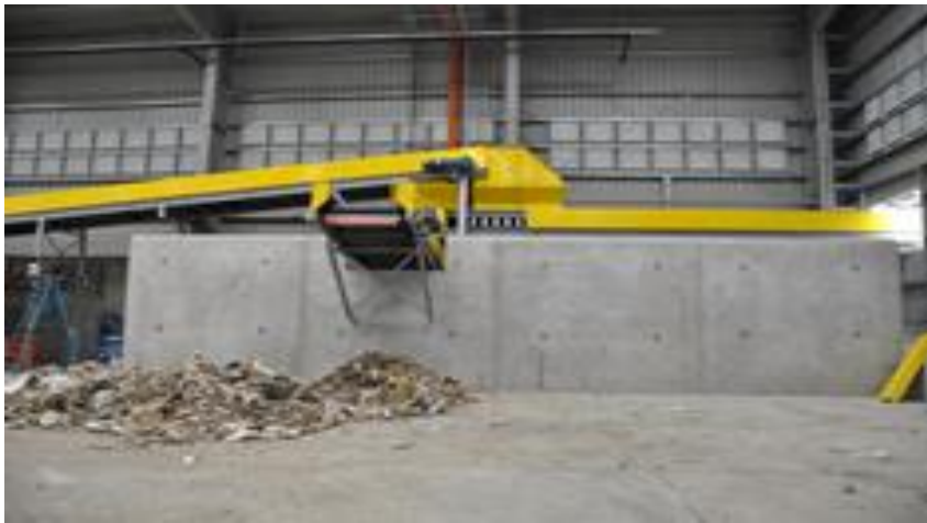
FIGURE 7 – PHOTO SHOWING RESIDUE WASTE BEING RE-CIRCULATED AND THEN DEPOSITED INSIDE THE MPC BUILDING
