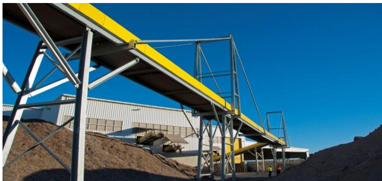
FIGURE 8 – PHOTO SHOWING THE CONVEYOR FROM THE WESTERN SIDE OF THE MPC BUILDING DESIGNED TO CARRY SMALL TIMBER PIECES TO THE WOOD WASTE STORAGE AREA, WHERE IT IS DEPOSITED INTO A STOCKPILE AND SUBJECT TO FURTHER SORTING
