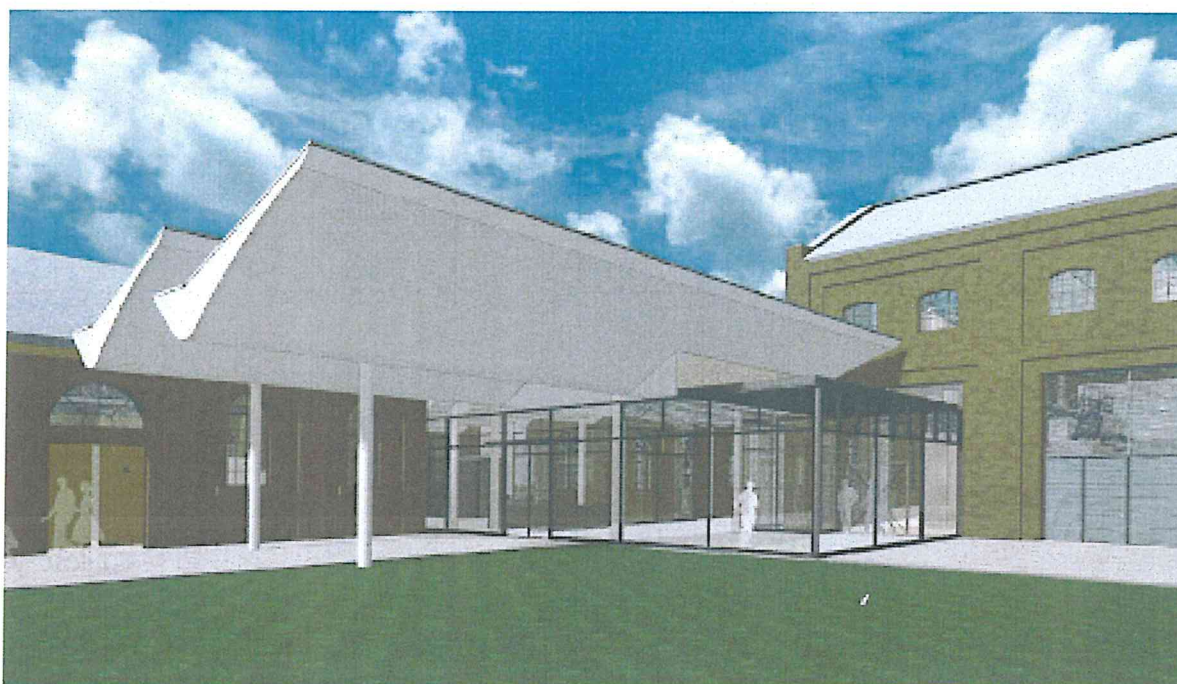
Figure 5 Perspective drawing of the proposed Link with its own sawtooth roof — FJMT
