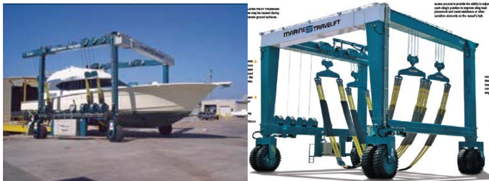
Figure 4-1 Examples of a travel lift in operation and how the slings hang when not in use (Source: marintavellift.com)
