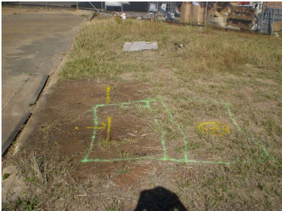
Photo 13- Localised staining observed in the vegetated area within proximity to the eastern site boundary (sample location TP17).
