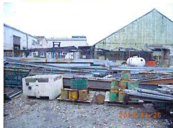
Photo # 149: Oil drums, containers, stored outside the workshop, filled with rain water. The green small drums were labelled as liquid emulsifier.
