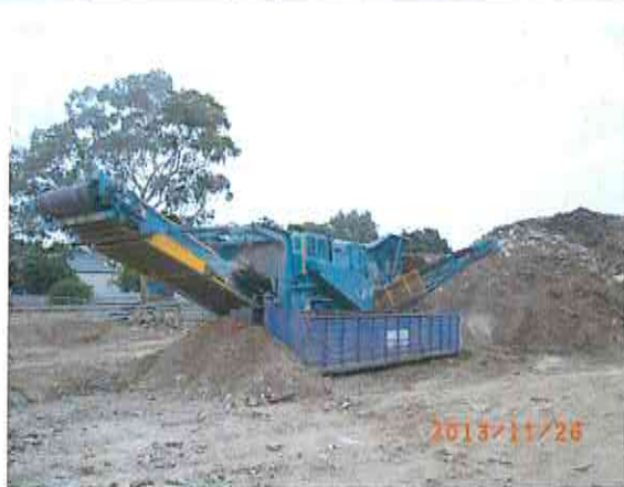
Photo # 217: Crusher and screening of C&D waste.
