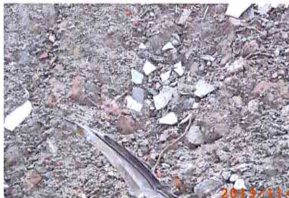
Photo # 009: Waste material (confirmed ACM) found in processed soil stockpile 4, refer to section 3.1.1 of discussion of laboratory results and Appendix B for laboratory report.
