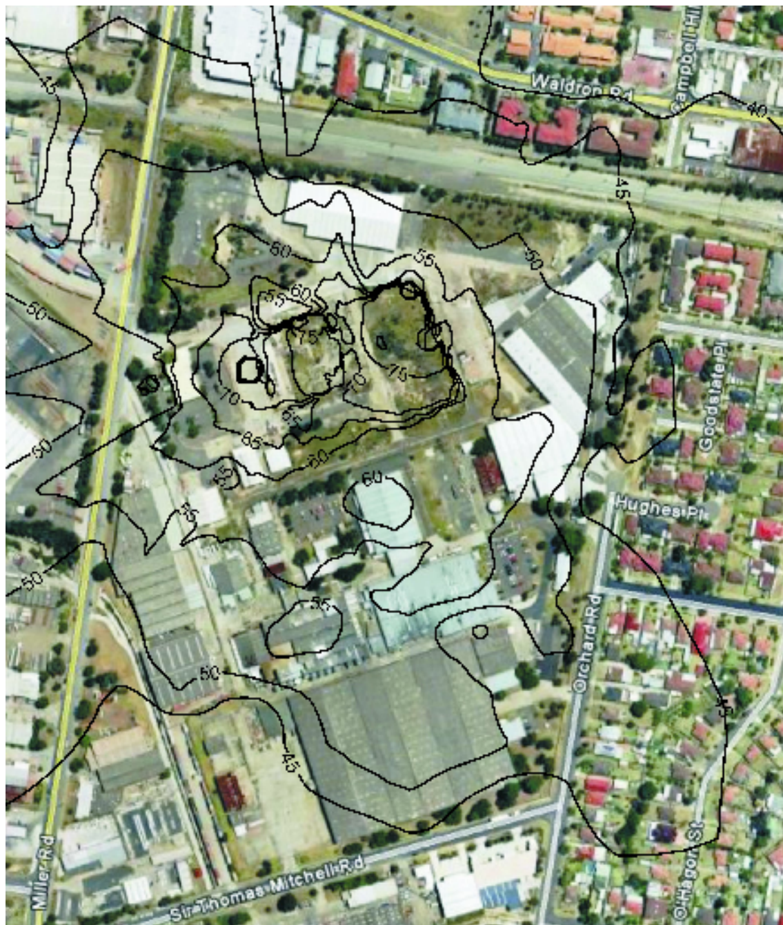
Figure 2. Predicted noise levels under a 4°C/100m temperature inversion.
