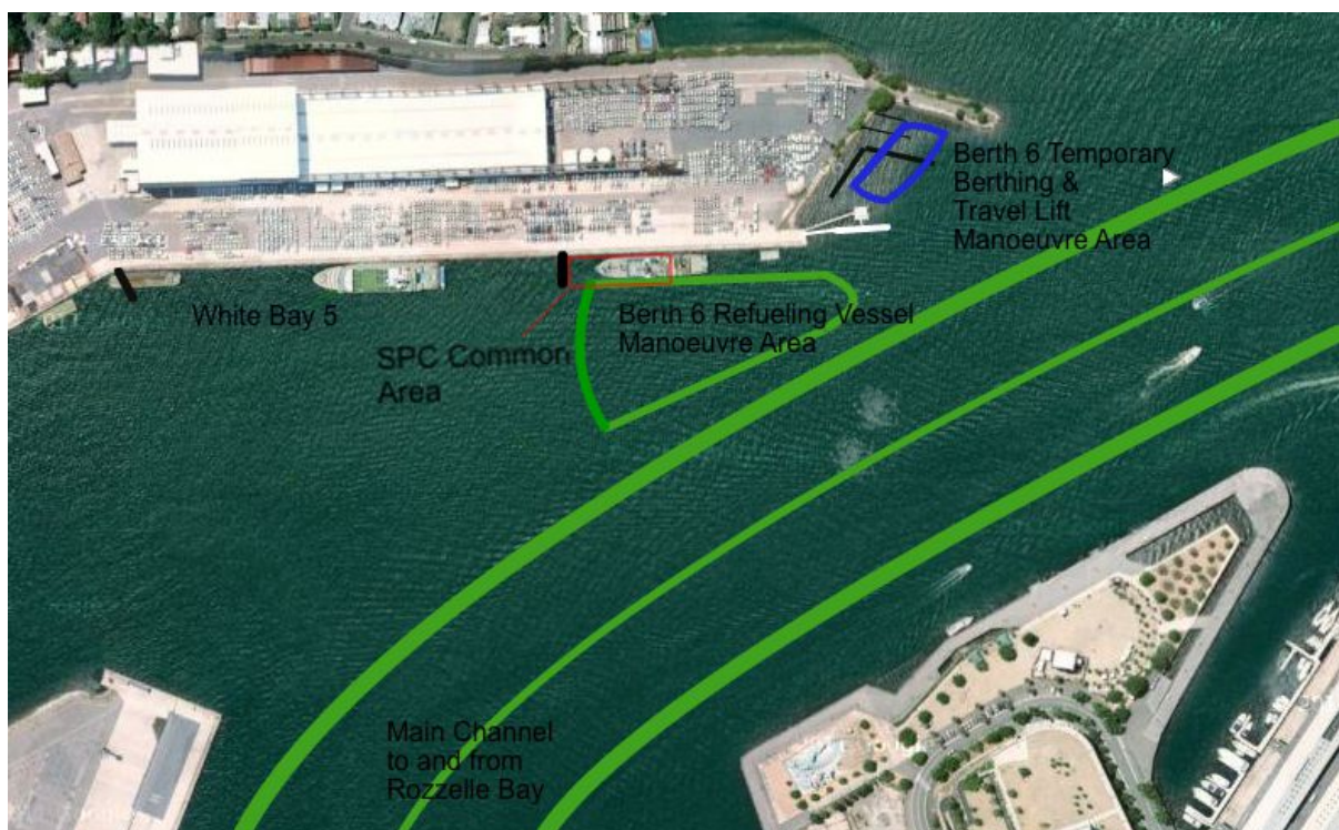
Figure 4. Indicates in blue the temporary berthing, RoRo and travel lift manoeuvre area. The SPC common area for berthing cruise ships is depicted in red. The Berth 6 refuelling vessel manoeuvre area as depicted in the Operational Environmental Management Plan is also included.
