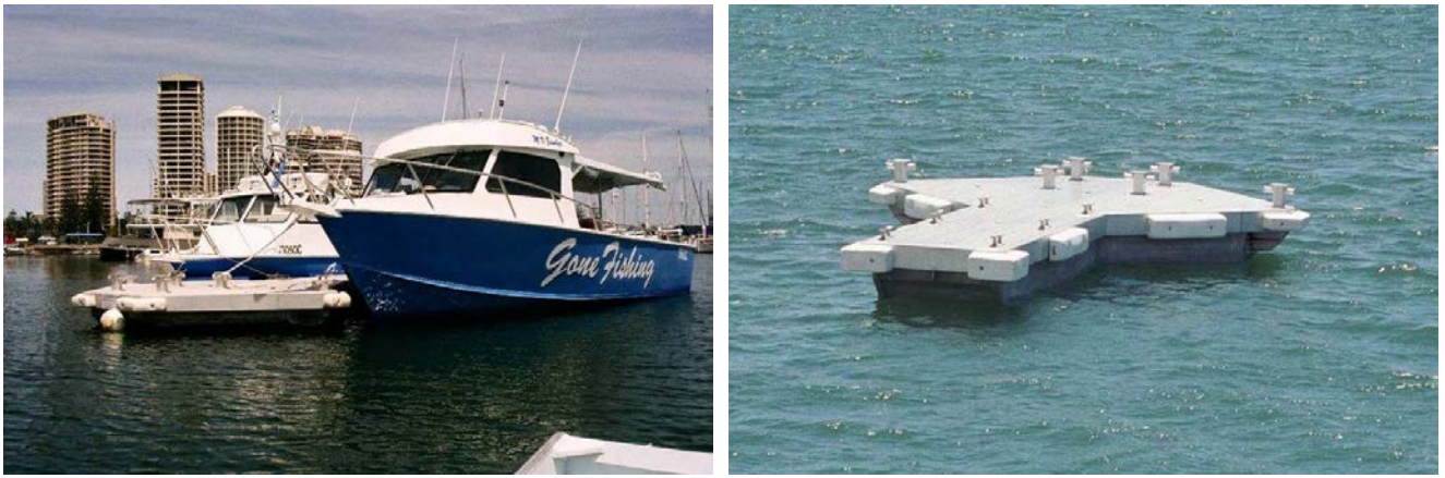
Fig. 29 & 30 - A pontoon mooring system showing vessels attached (29) and the system (30)
