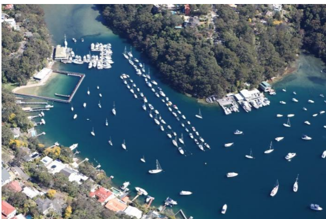
Fig. 27 - Fore and aft moorings, berths and scattered moorings
