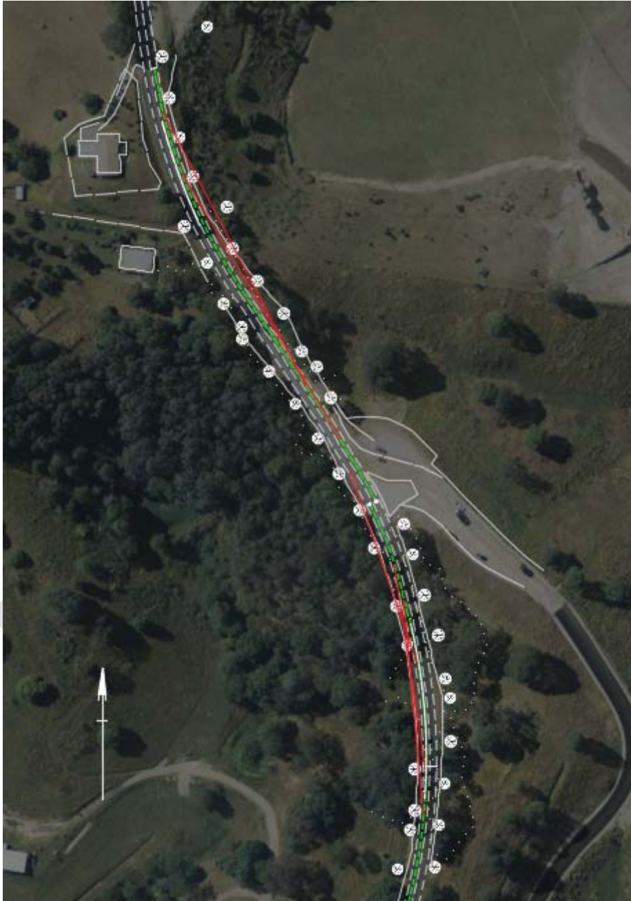
Figure 2: Preliminary SSD check showing absolute minimum design parameters (red lines)
