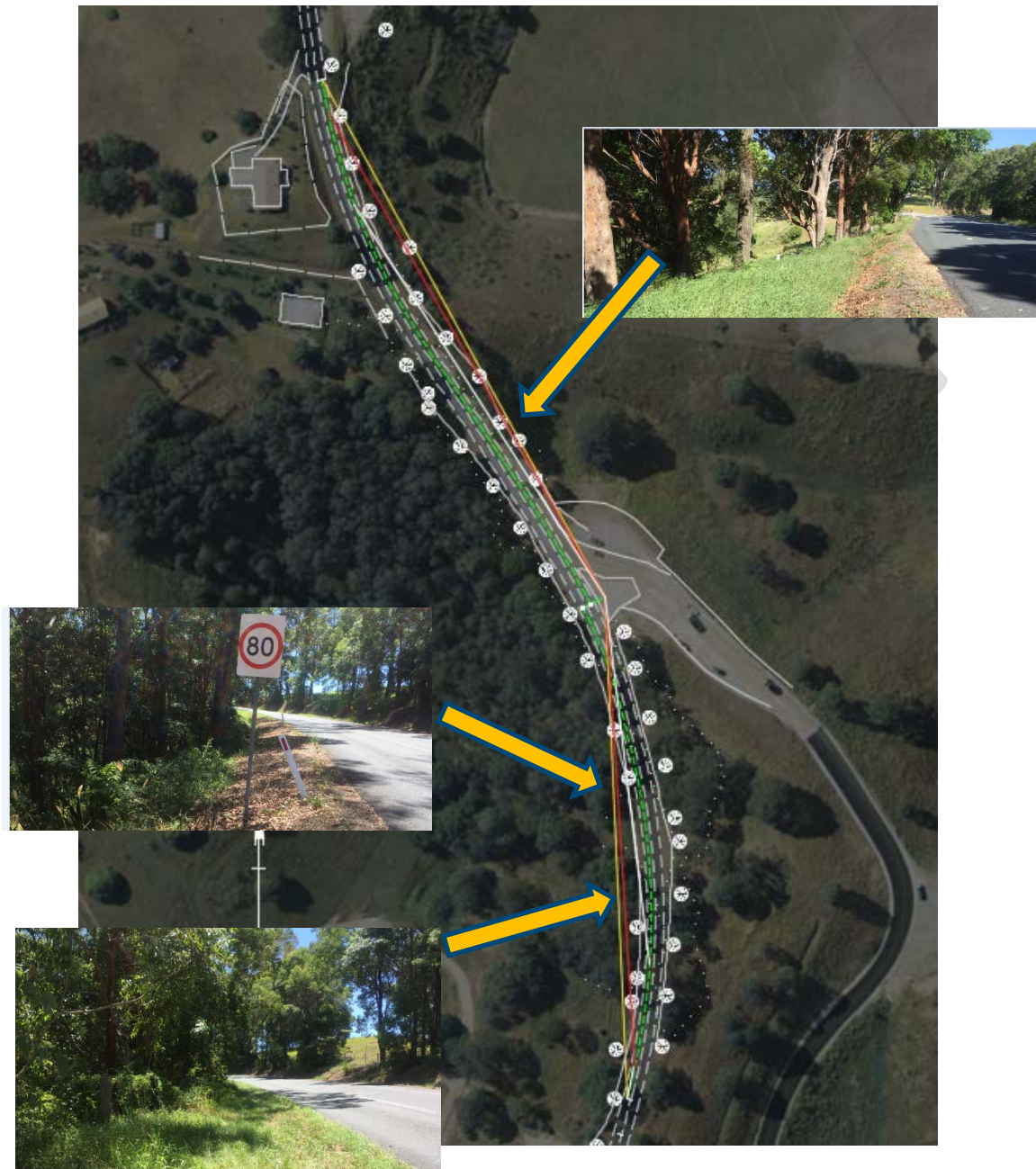
Figure 3: Preliminary SISD check showing absolute (red lines) and preferred (yellow lines) minimum design parameters
