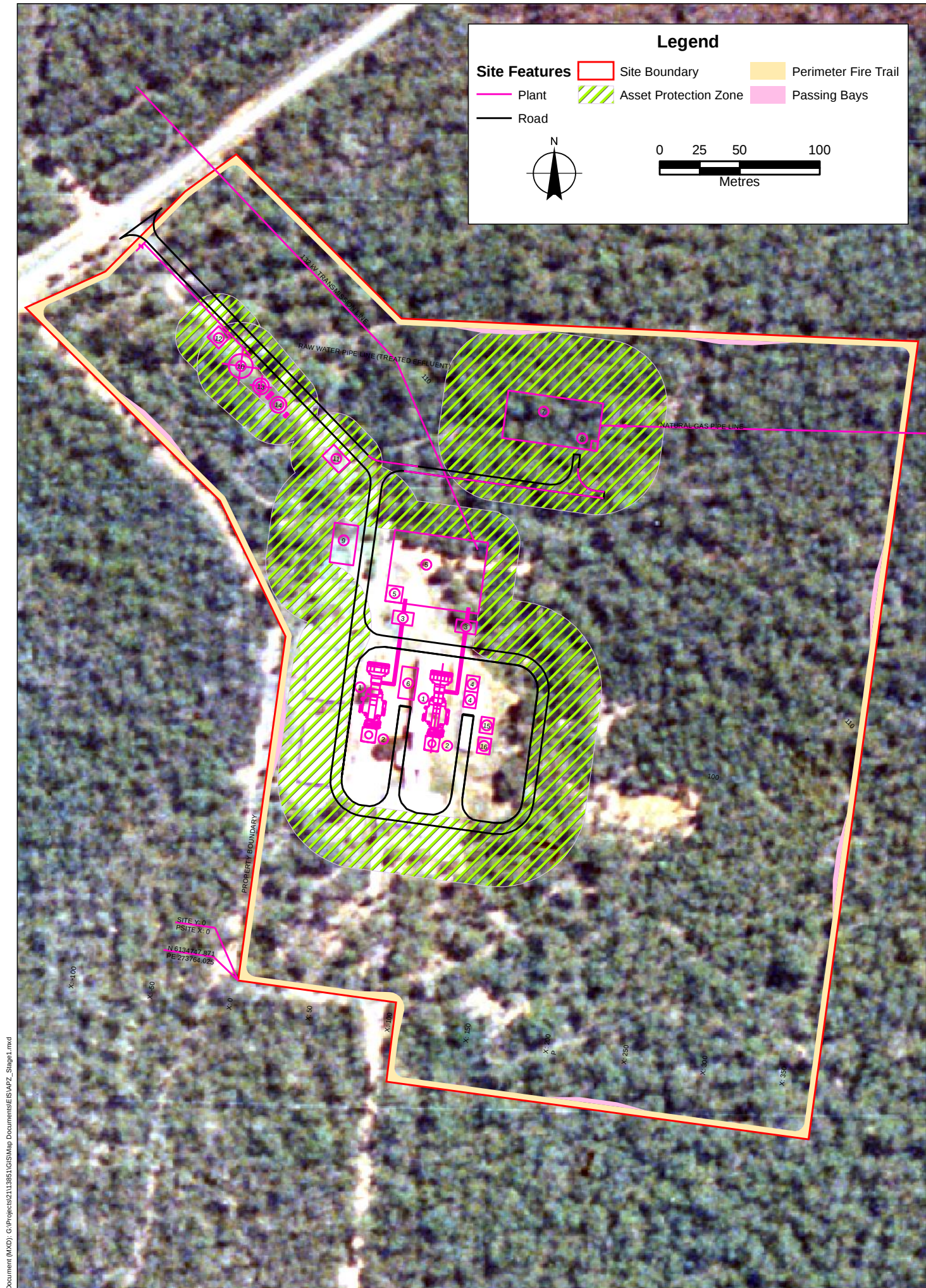
Figure 4 - Fire Protection Requirements (Stage1)
