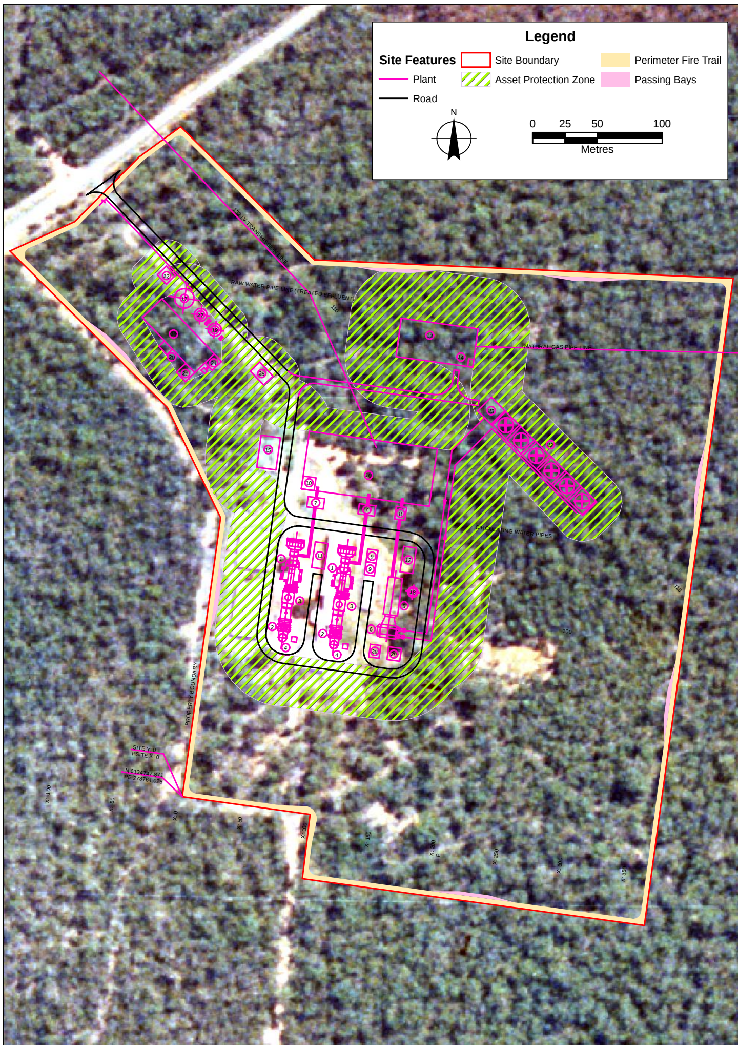
Figure 5 - Fire Protection Requirements (Stage 2)
