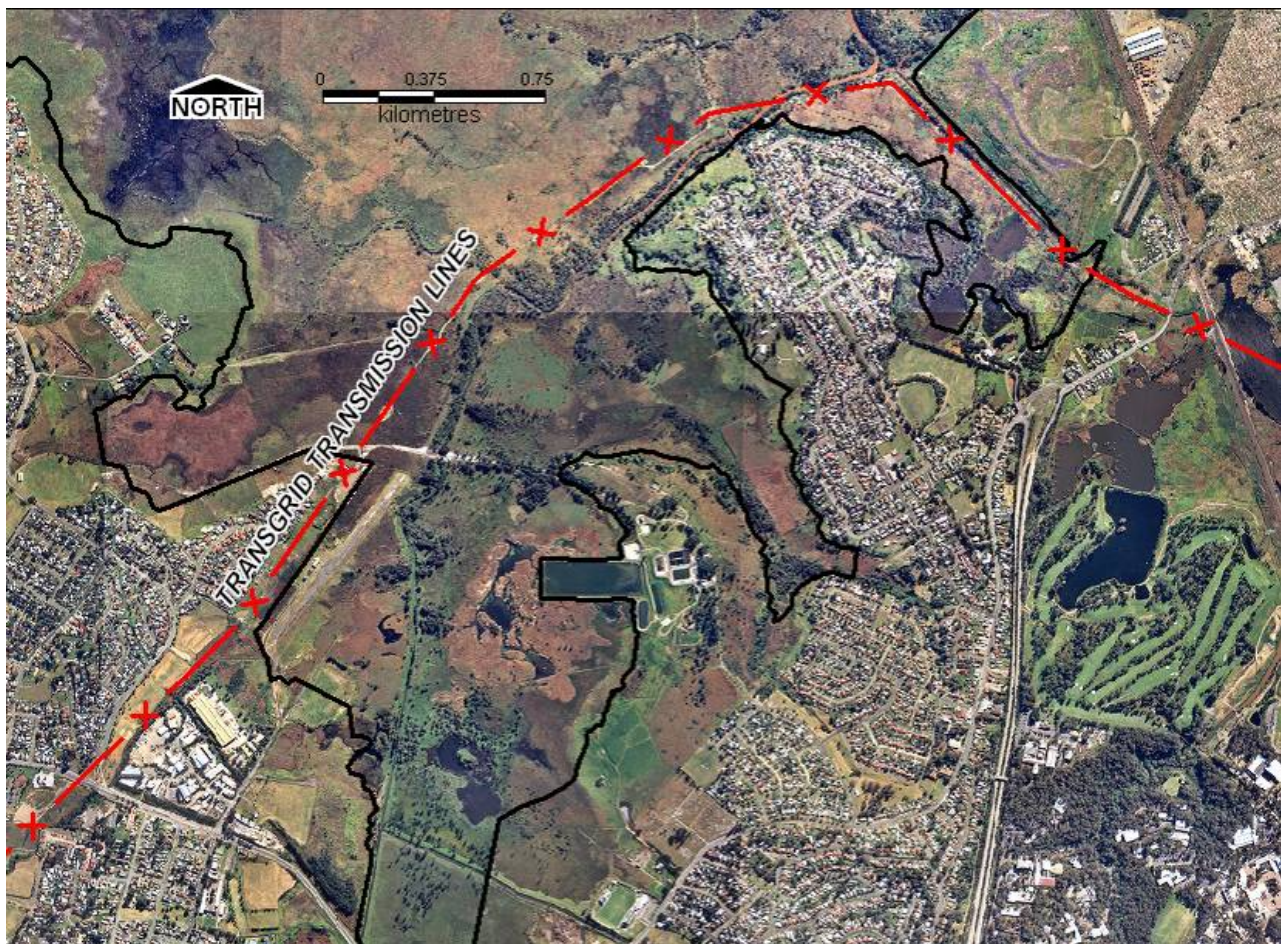
Figure 3.23 Location of Transgrid Transmission Lines across Hexham Swamp
