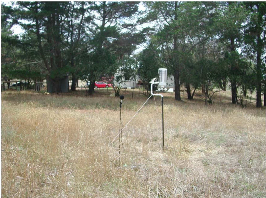
Site 8: Noise Monitor Set-up and Location relative to Residence and Property.
