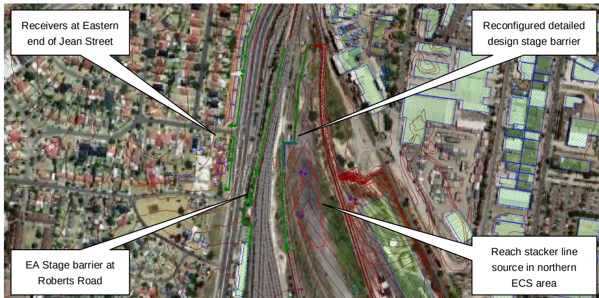
Figure 4-3 – Roberts Road barrier reconfiguration
