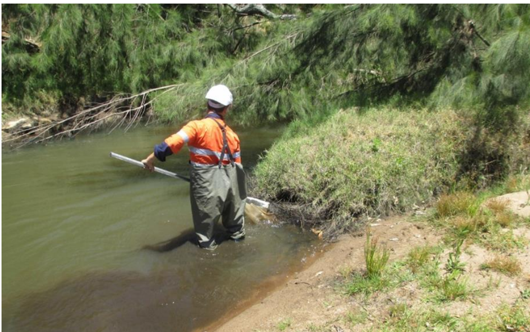
Plate 1: Sampling method – dip netting
