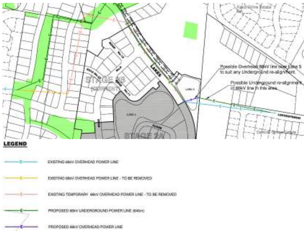
Figure 75 - Proposed Option 1 for underground re-routing existing 66KV electricity supply (Source: Resource Design Management 2007)
