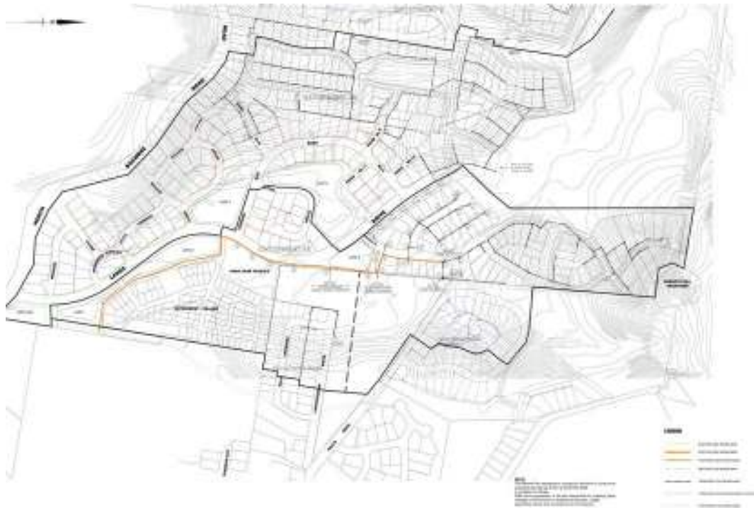
Figure 72 – Reticulated sewer strategy for Catchment 1A and 1B (Source: Resource Design Management 2007)
