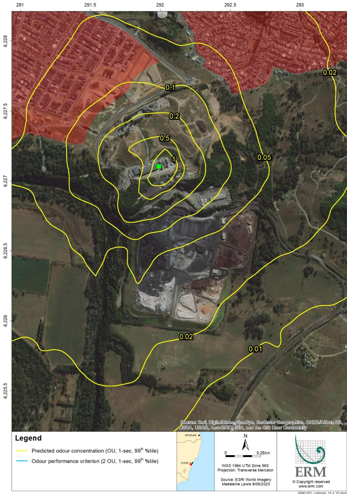
Figure 7-3: Predicted 99 th percentile ground level odour concentration for grease trap waste only
