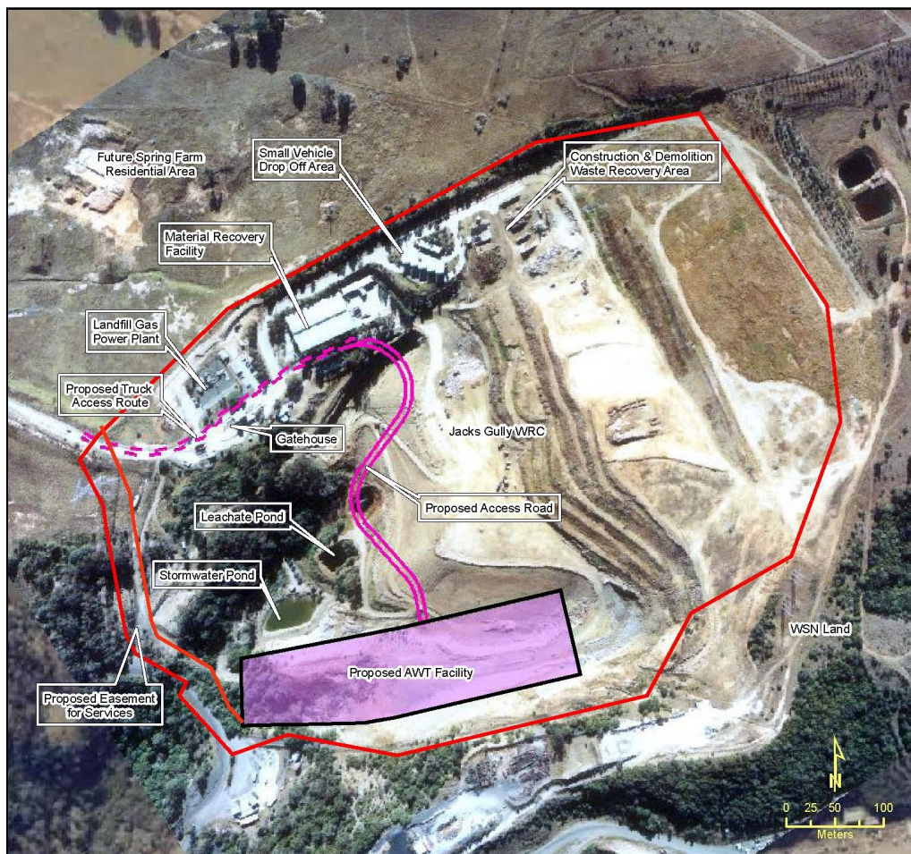
Figure 2.1: Layout of Jacks Gully WMC site
